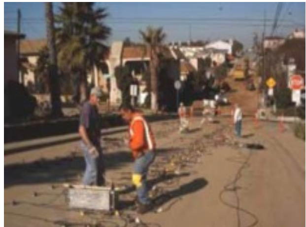
Crew performing seismic survey using "MicroVib" vibration source box
