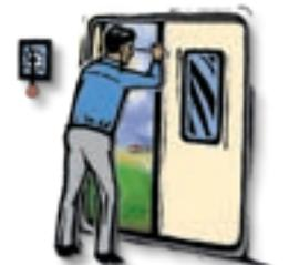
To exit through the emergency windows, pull the red handles toward you. Remove the window by pulling it toward you using both
