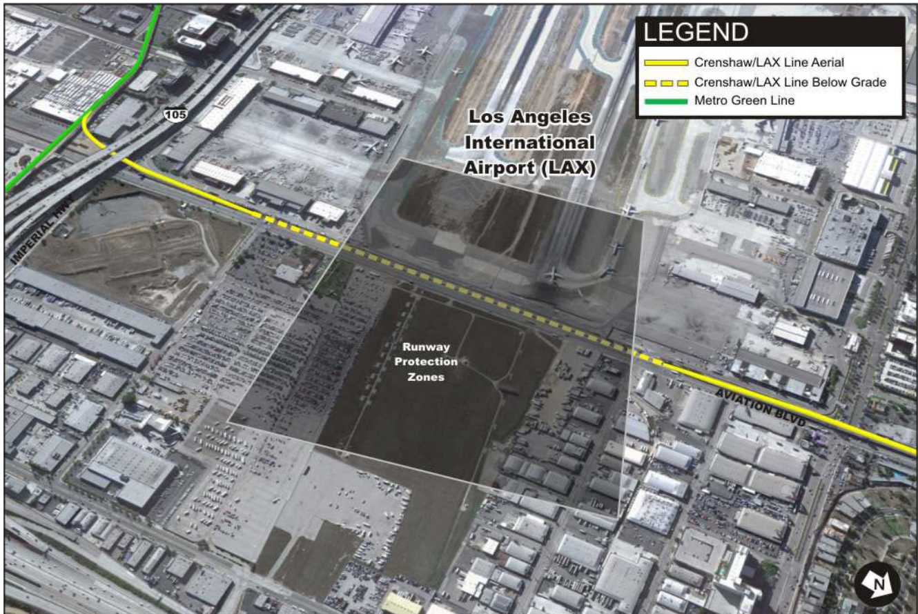
Below-grade trench alignment along Aviation Boulevard, adjacent to LAX south runways.
