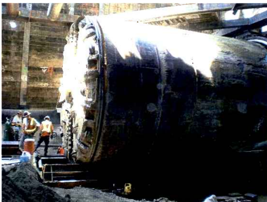
Eastbound Tunnel Boring Machine at Soto Station.
