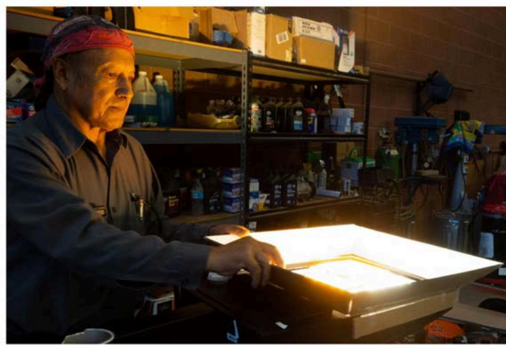
Ivins Fleet Mechanic Wilson Jimenez fits a shield onto his light-filter prototyping station in the city garage. He designed the amber insert that adapts the city's LED bulbs to be "night sky friendly" and has custom-built about 150 inserts to date.
