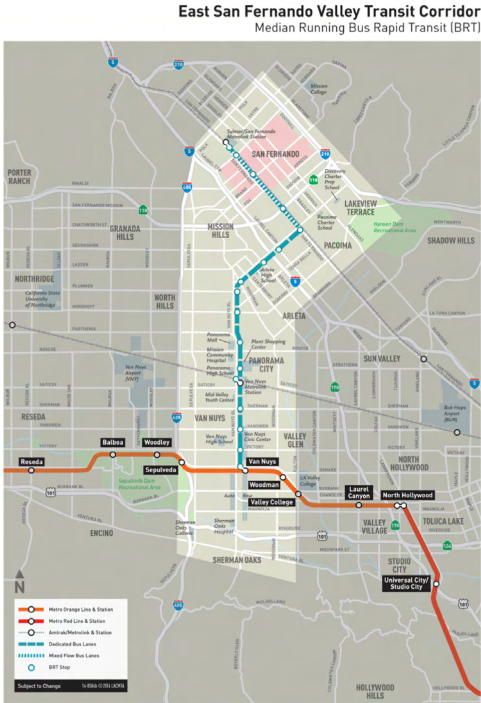
Figure 1-3: Build Alternative 2 – Median-Running BRT Alternative
