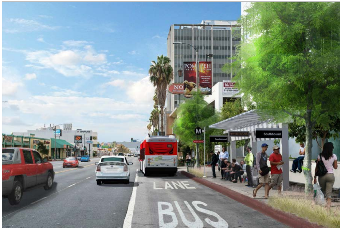
Figure 4-2: Architectural Rendering for Curb-Running BRT Alternative
