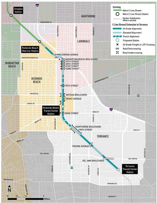
Figure ES-15. Overview of 170th/182nd Grade-Separated Light Rail Transit Alternative
