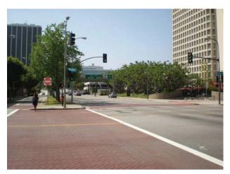
Photo 4 - The Flower Street and 3<sup>rd</sup> Street intersection has excellent sight distance and is very open. The east leg begins the uphill grade to Bunker Hill.
