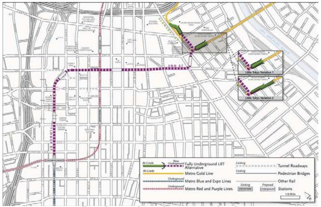
Figure 5-5. Fully Underground LRT Alternative – Little Tokyo Variation 1
