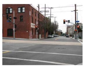
Photo 26 – I<sup>st</sup> Street and Main Street exhibits marked pedestrian crosswalks on three legs. Pedestrian crossing is prohibited along the east leg.
