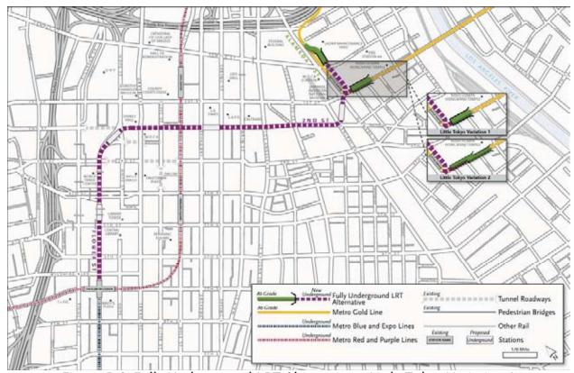
Figure 5-6. Fully Underground LRT Alternative – Little Tokyo Variation 2
