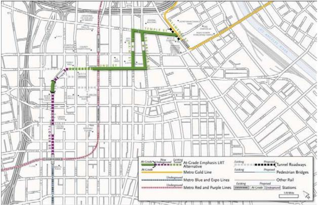
Figure 5-3. At-Grade Emphasis LRT Alternative
