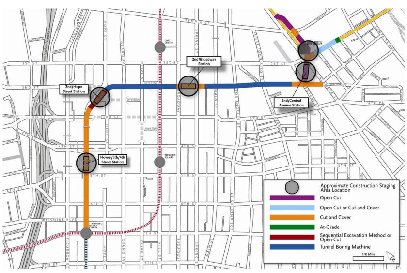
Figure 4-2C Construction Methods (Fully Underground LRT Alternative)
