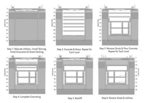
Figure 4-3. Cut and Cover Construction Method
