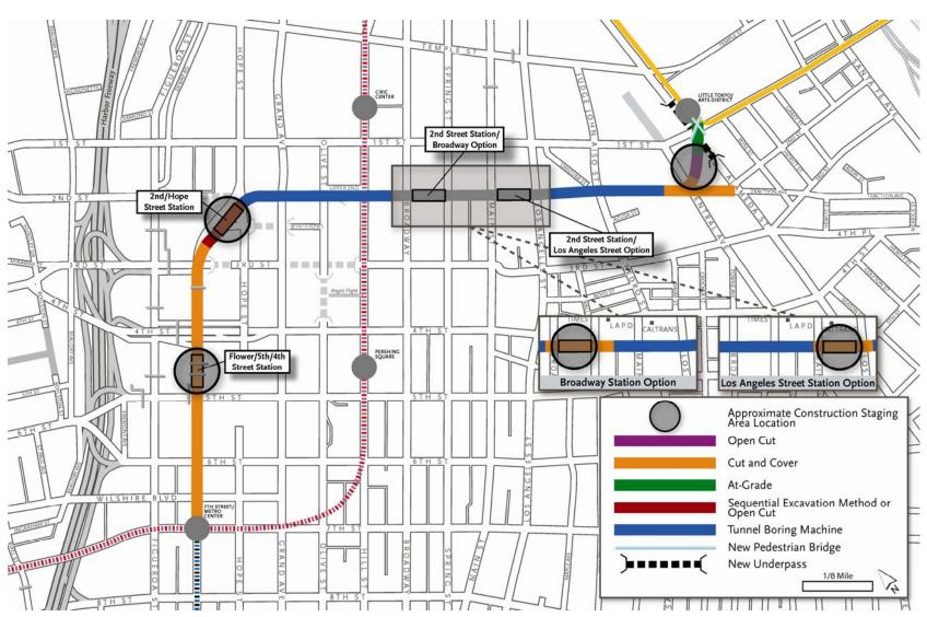
Figure 4-2B Construction Methods (Underground Emphasis LRT Alternative)
