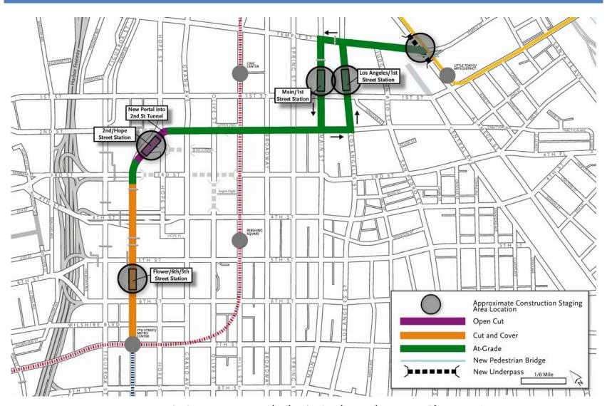
Figure 4-2A Construction Methods (At-Grade Emphasis LRT Alternative)
