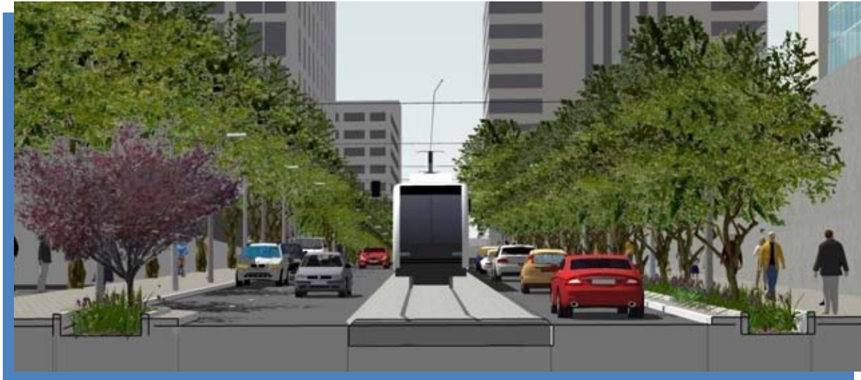
Figure 2-4. Typical At-Grade Alignment
