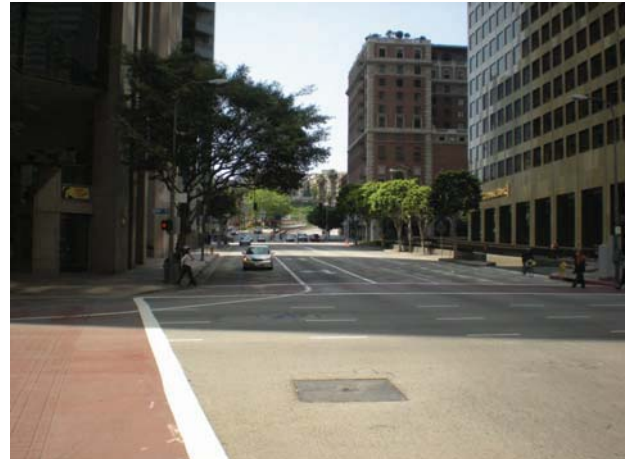
Photo 1 - The west leg of 6th Street carries one-way traffic from SR 110. Vehicle speeds were observed in the field to be higher than would be expected in a downtown environment.
