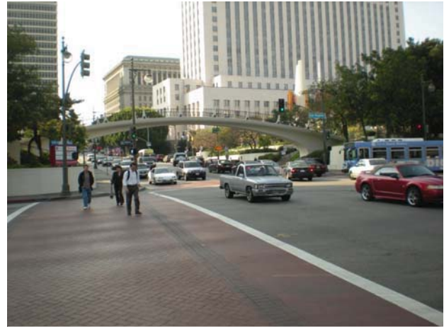
Photo 19 – The intersection of Temple Street and Los Angeles Street is adjacent to City Hall. Vehicle queuing was observed to back up into pedestrian crosswalks during peak time – a potential safety concern.
