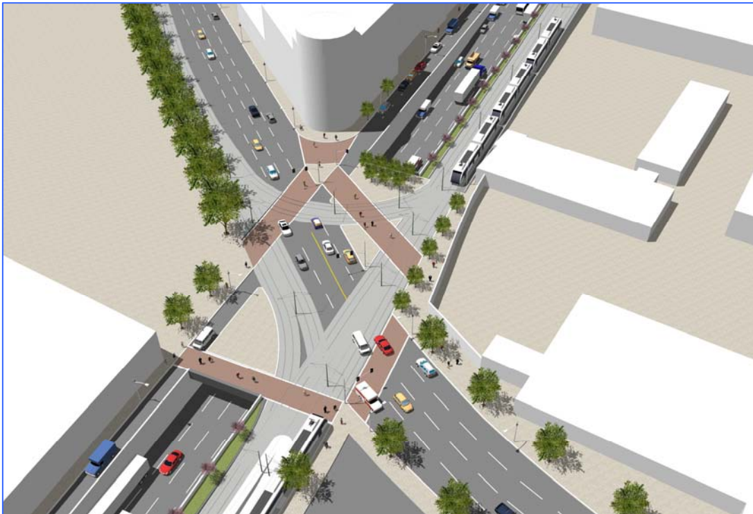
Figure 2-24 At-Grade Emphasis LRT Options A & B – Alameda St. Underpass at Temple and Alameda Streets Intersection
