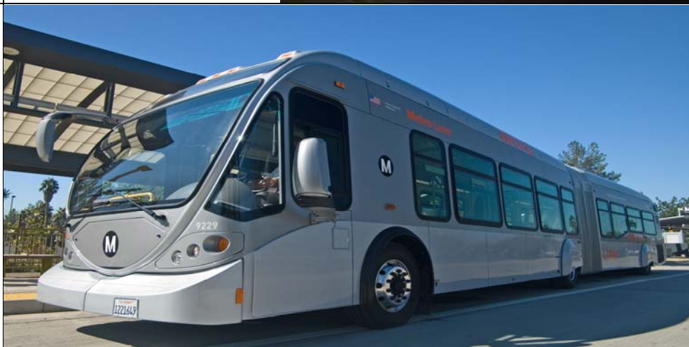
A BRT bus (Metro Orange Line) operating on dedicated right-of-way in an at-grade configuration
