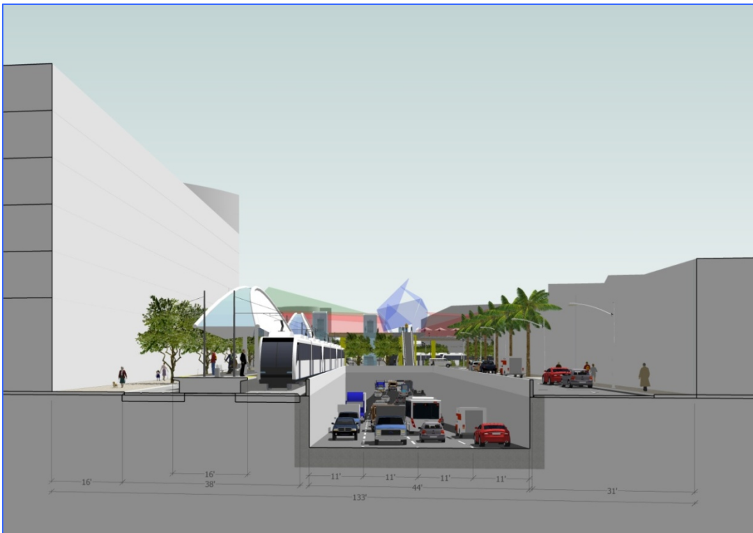
Figure 2-52 Underground Emphasis LRT Alternative – Alameda St. Underpass Looking South on Alameda St.
