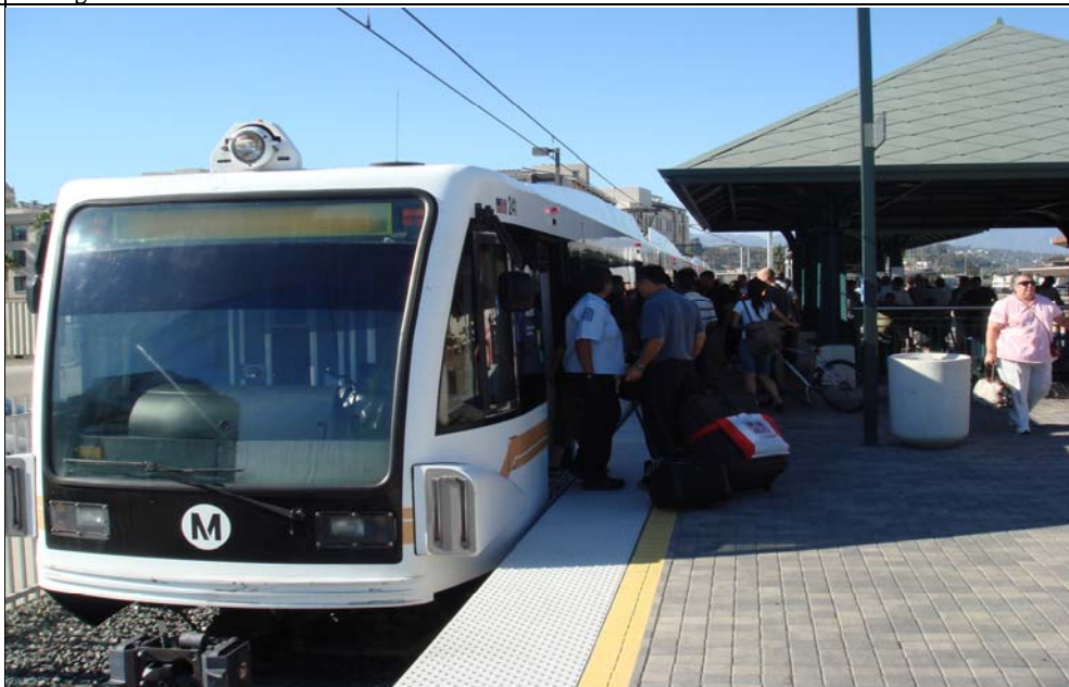
LRT train (Metro Gold Line) operating in an at-grade configuration
