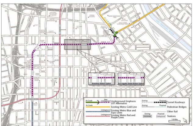
Figure 2-4. Underground Emphasis LRT Alternative Alignment and Configuration
