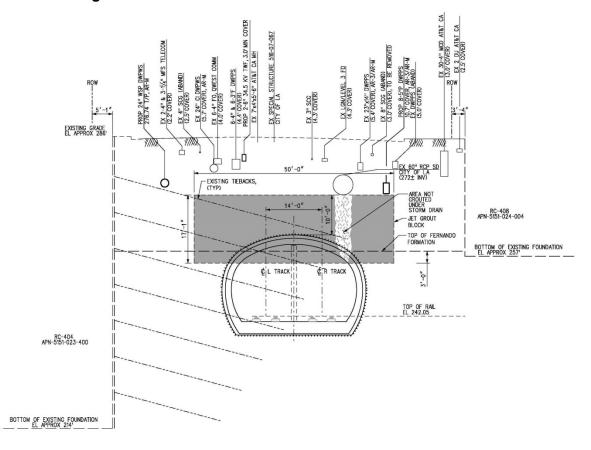
Figure 4-9: Jet Grout Zone above SEM Tunnel on Flower Street
