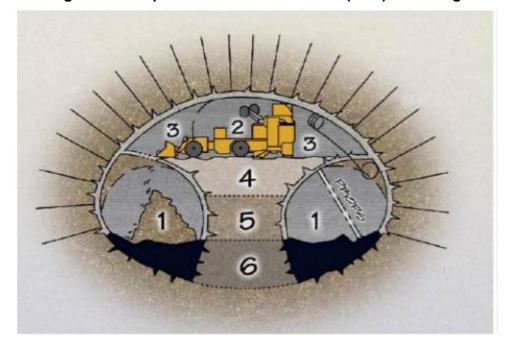
Figure 4-2: Sequential Excavation Method (SEM) Tunneling
