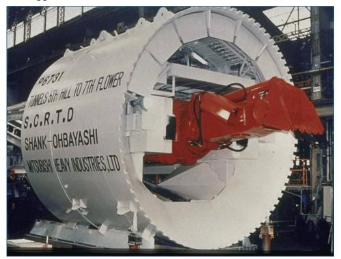
Figure 4-1: Digger Shield Used to Construct Metro Red Line Contract A146 Tunnels
