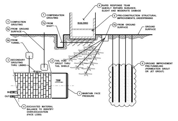
Figure 4-3: Grouting Methods for Tunneling
