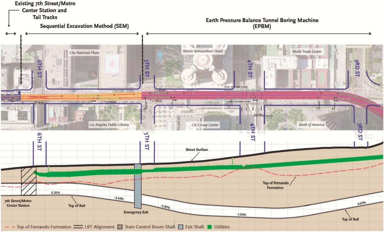
Figure 5-4: EPBM/SEM Low Alignment Alternative (Alternative B)
