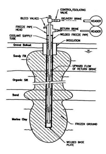
Figure 4-10: Individual Freeze Pipe Arrangement
