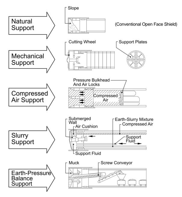
The cylindrical shield provides ground support and permits safe installation of a tunnel lining. Open-face shield tunneling is discussed in Section 4.3 of this report. Closed-face tunnel shields
