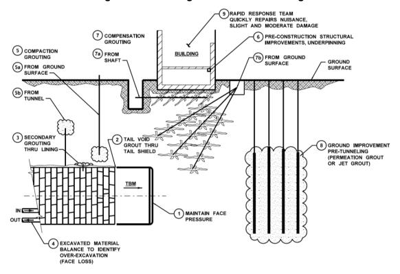
Figure 4-3: Grouting Methods for Tunneling
