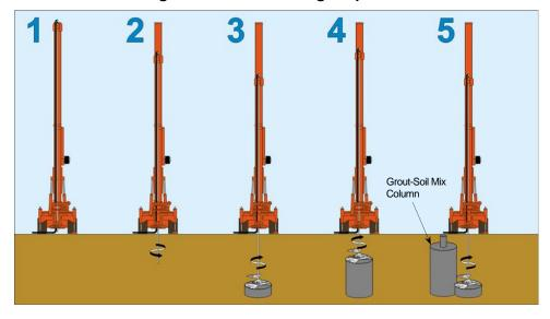
Figure 4-5: Jet Grouting Sequence
