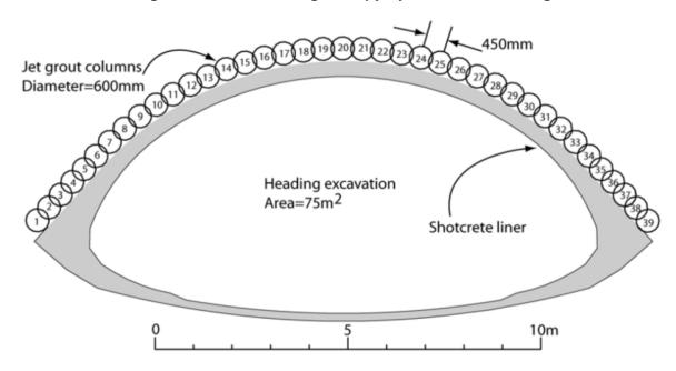
Figure 4-6: Jet Grouting Canopy by Horizontal Drilling
