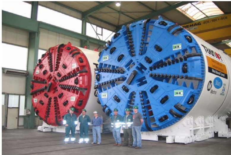
Figure 2.2-7: EPBMs Used for Construction of Los Angeles Eastside LRT Tunnels
