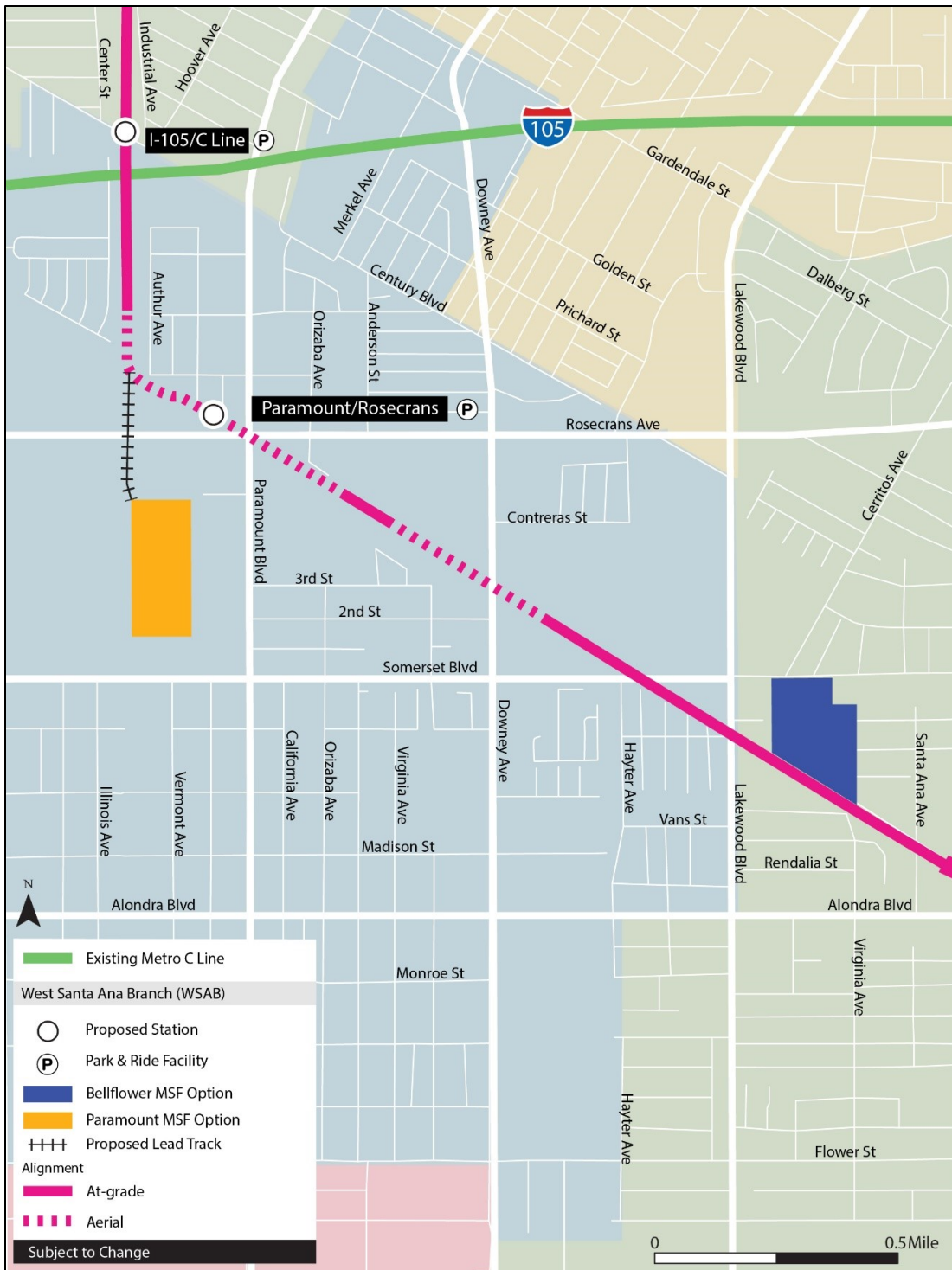
Figure 2-7. Maintenance and Storage Facility Options
