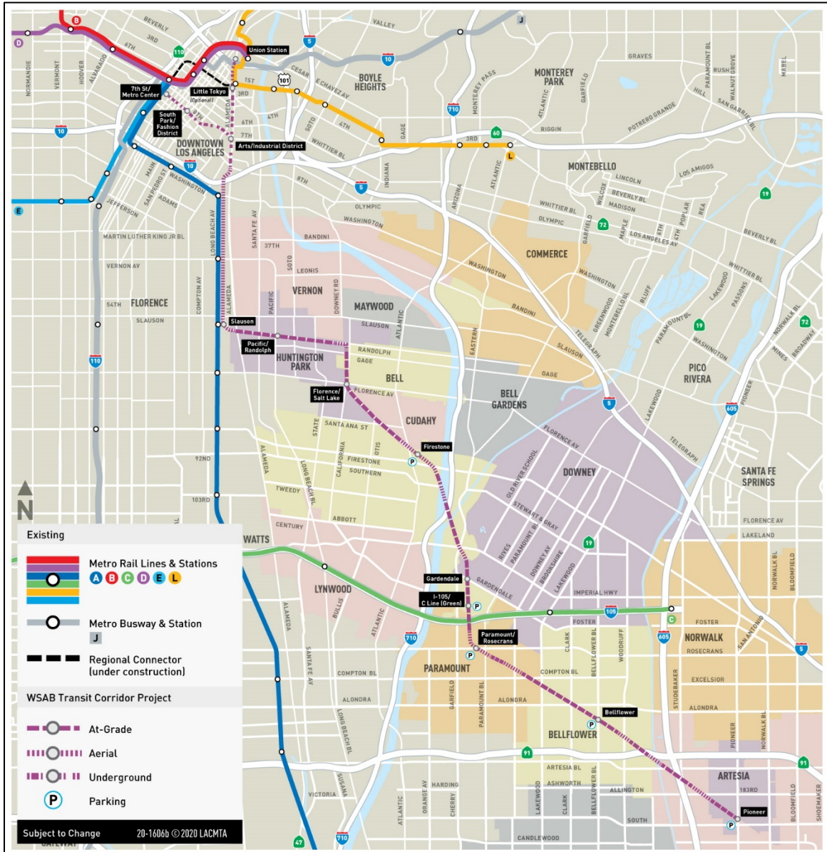
Figure 2-2. Project Alignment by Grade
