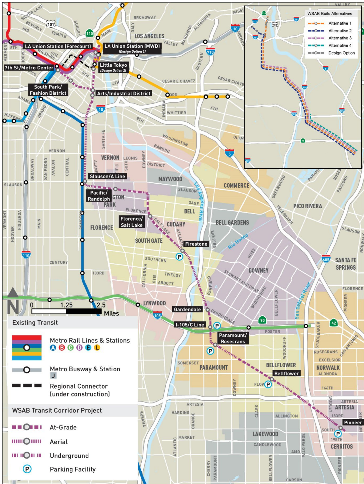
Figure 2-2. Project Alignment by Alignment Type
