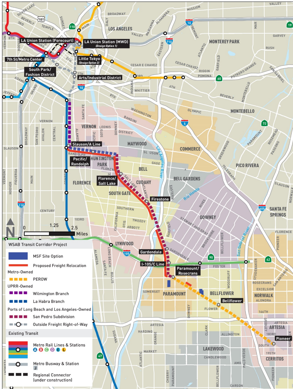
Figure 2-6. Existing Rail Right-of-Way Ownership and Relocation
