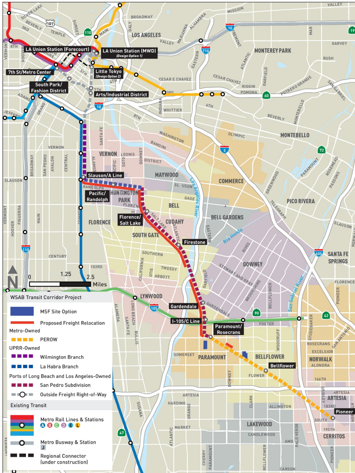
Figure 2-6. Existing Rail Right-of-Way Ownership and Relocation
