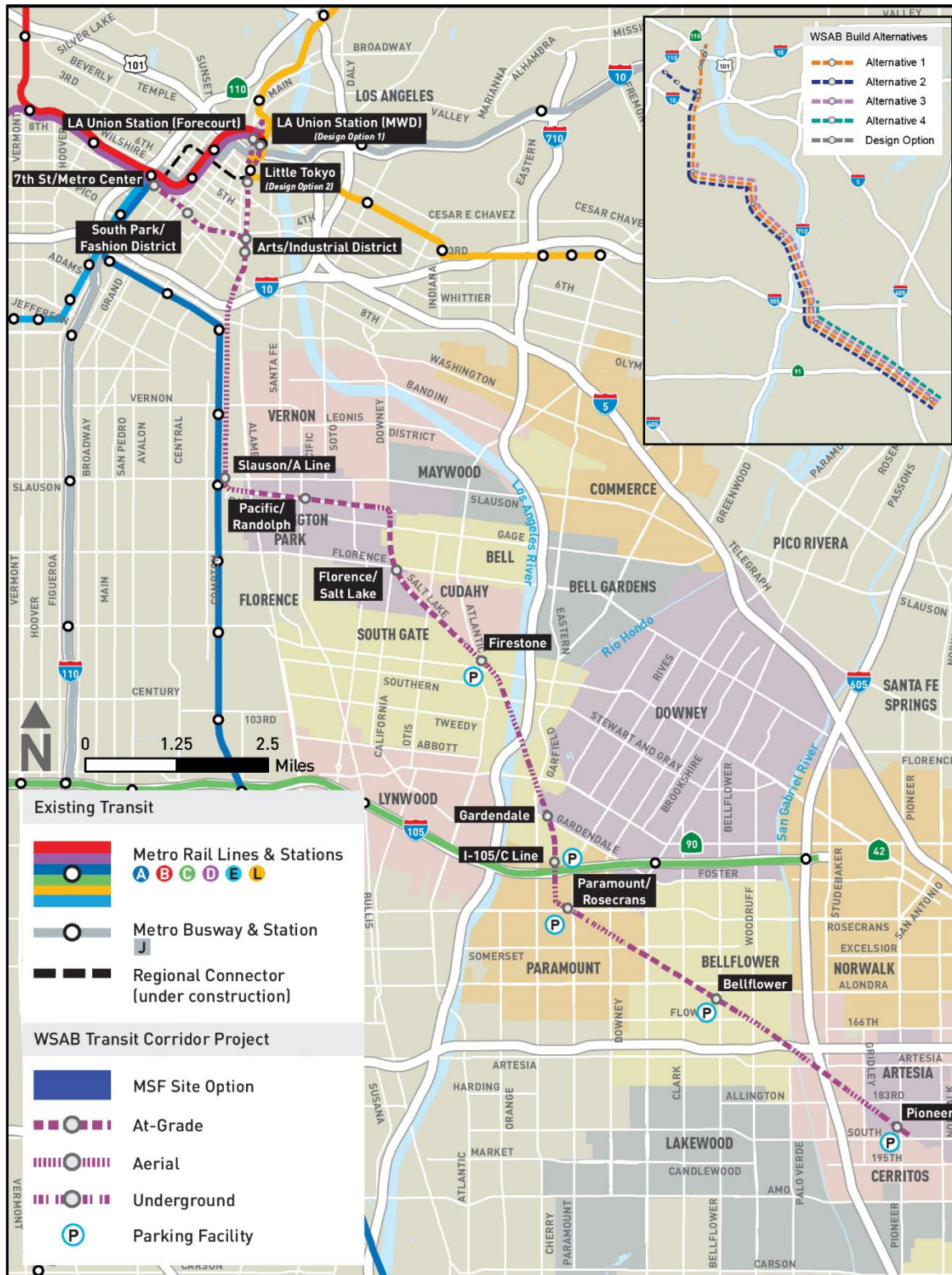
Figure 2-2. Project Alignment by Grade
