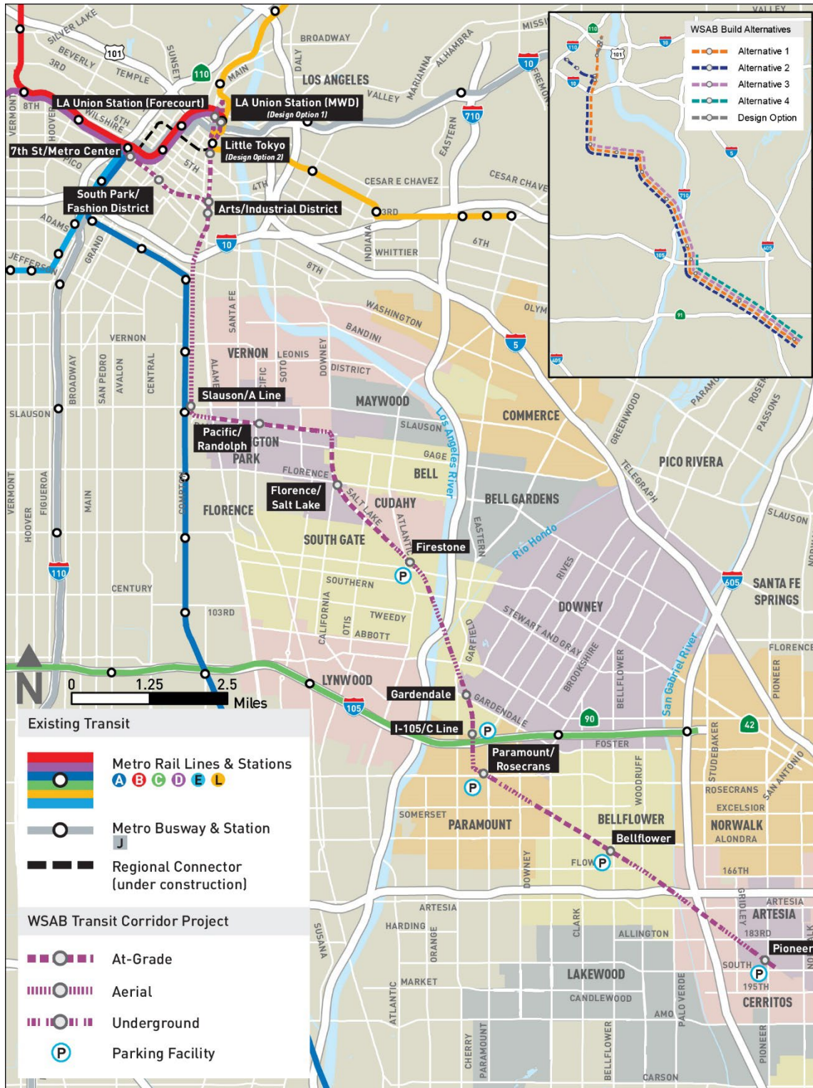
Figure 2-2. Project Alignment by Grade
