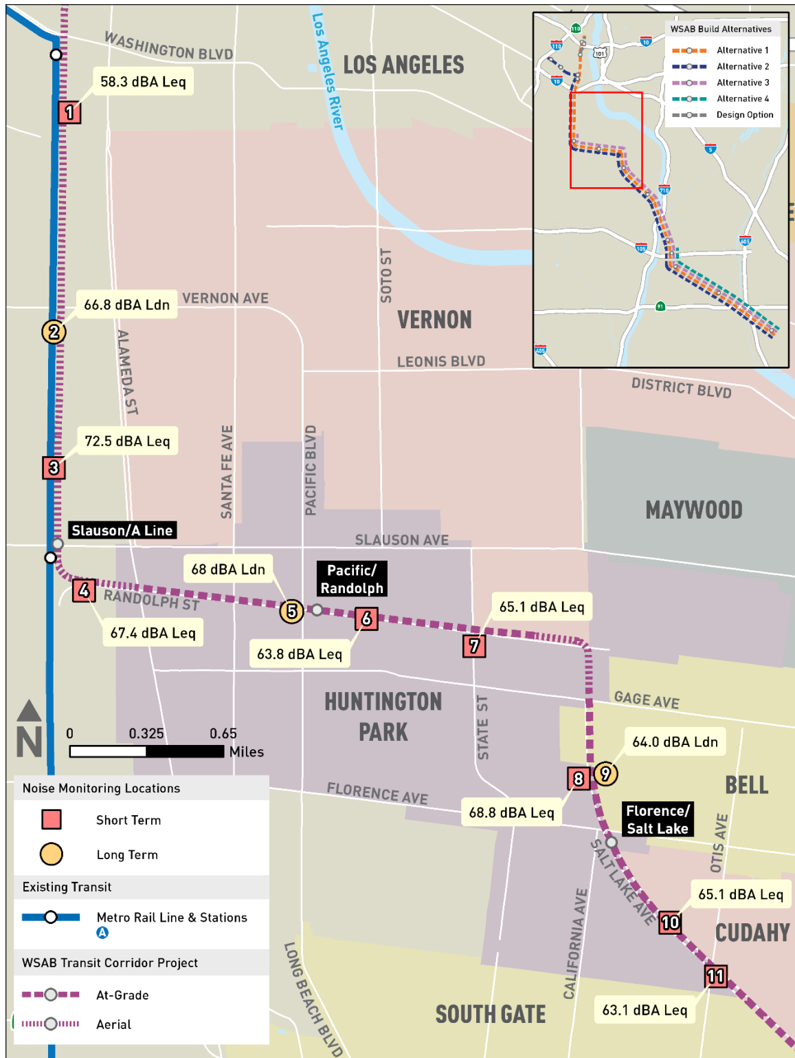
Figure 4.7-2. Noise Monitoring Locations and Existing Noise Levels
