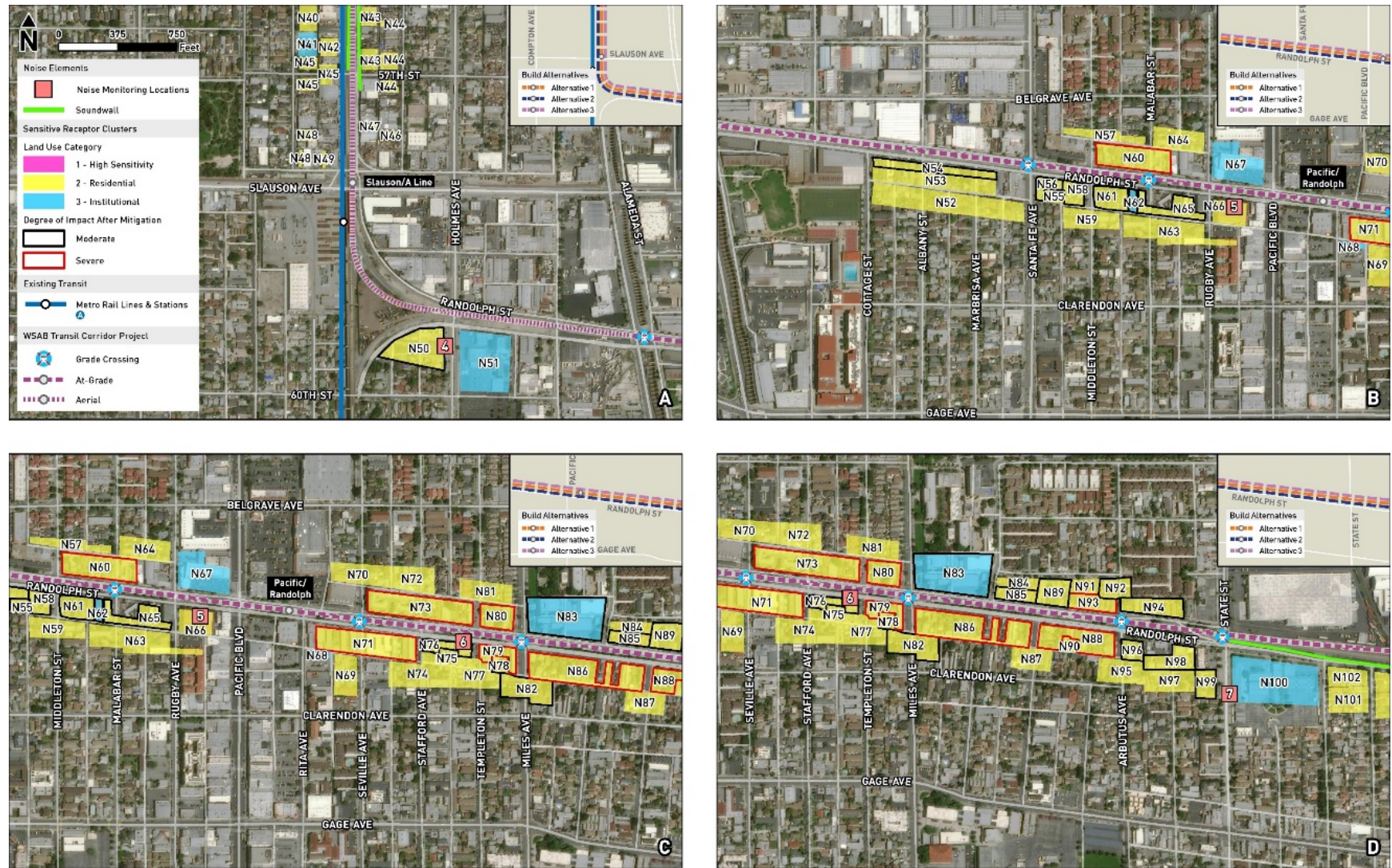
Figure 4.7-6. LRT Noise Impacts Remaining After Mitigation, including Soundwalls (Florence to City of Huntington Park)
