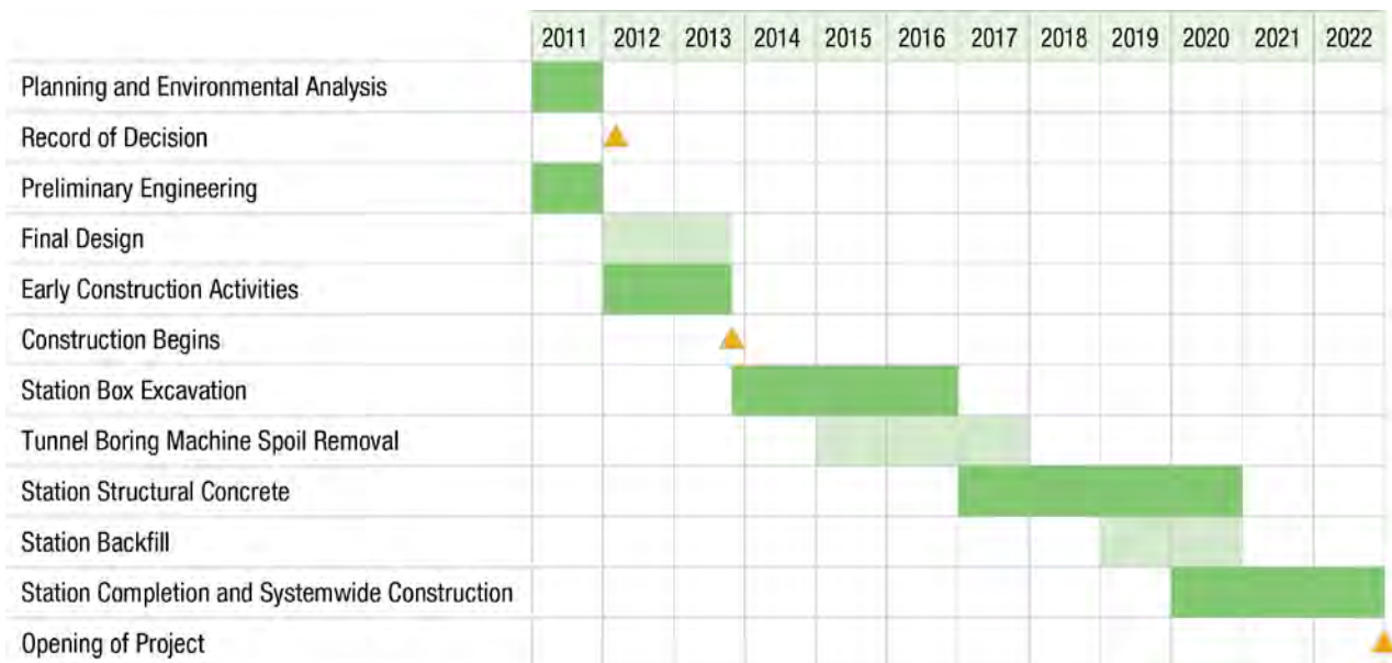
Figure 4-66. Construction Schedule under Concurrent Construction Scenario
