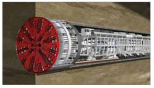
Figure E-3. Typical Tunnel Boring Machine
