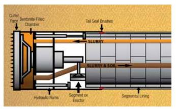
Figure E-13. Slurry Face TBM
