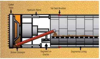
Figure E-12. Schematic of EPB TBM
