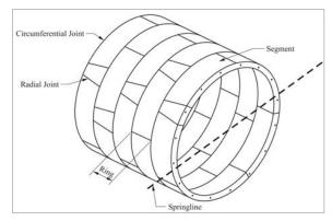
Figure E-16. Typical Precast Concrete Segmental
