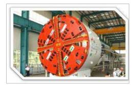
Figure E-8. Typical Pressurized-Face TBM
