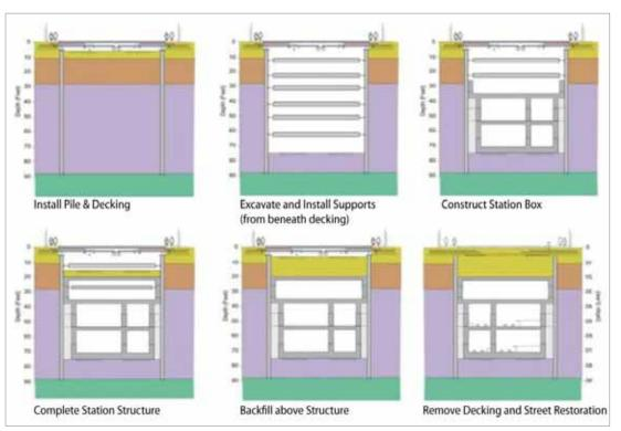
Figure E-4. Typical Cut-and-Cover Construction Sequence
