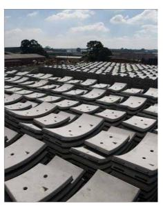
Figure E-17. Precast Concrete Segments Storage
