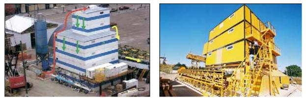
Figure E-15. Slurry Treatment Facilities (Stacked Configuration)
