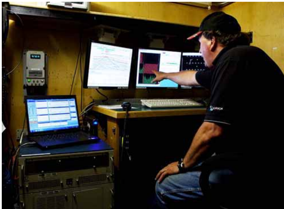
Figure 3 Aries/ARAM II Seismic Acquisition System
