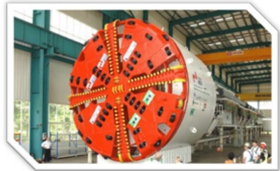
Figure 4-9: Typical Pressurized-Face TBM
