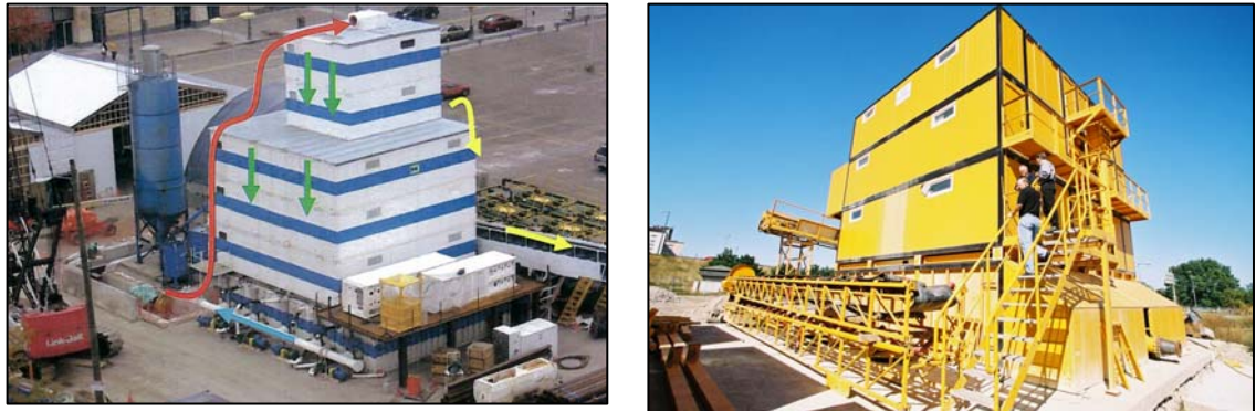
Figure 4-21: Typical Slurry Treatment Facilities (Stacked Configuration)
