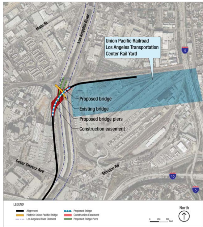
Figure 2-15: UP Railroad Rail Bridge
