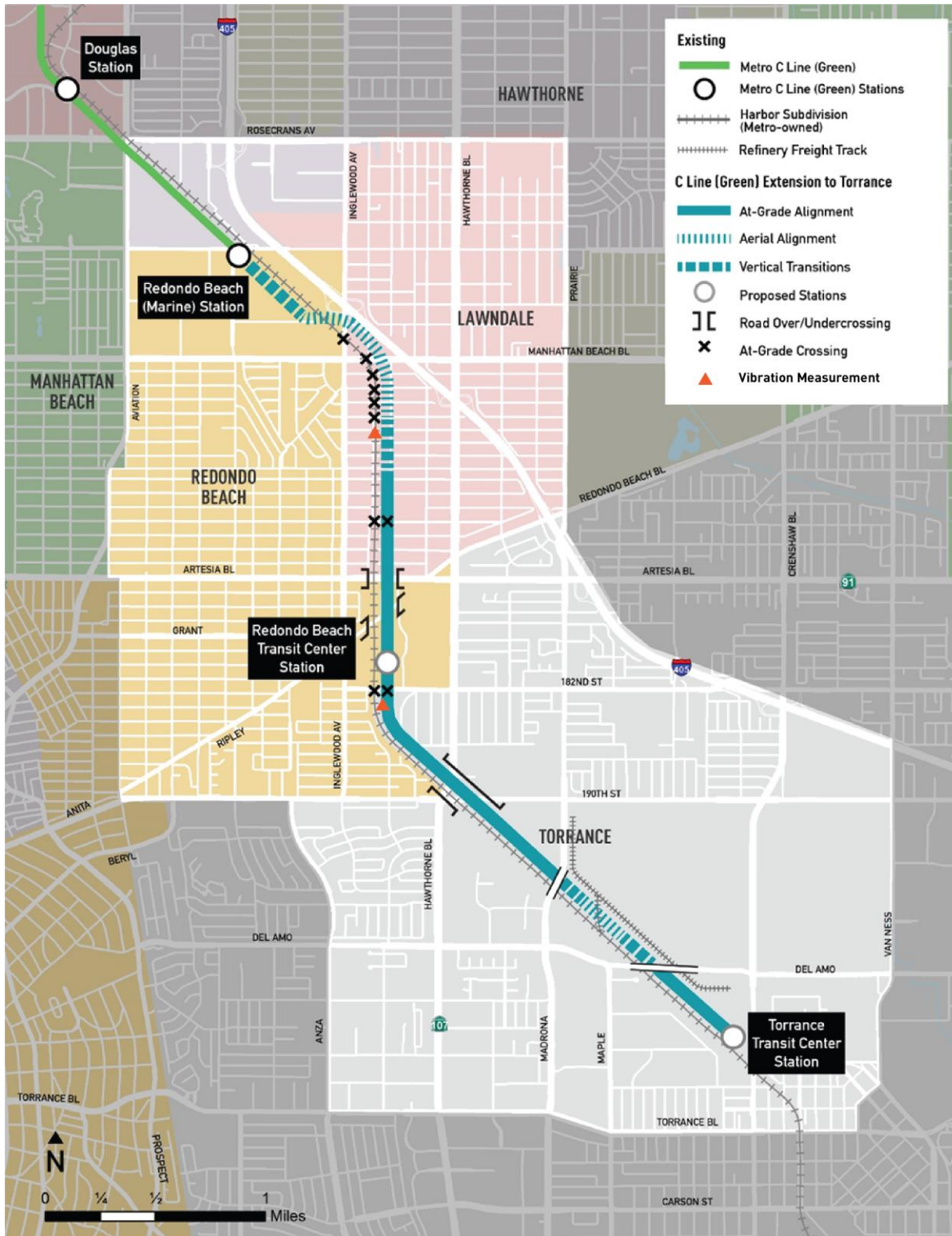
Figure 3.6-9 Vibration Measurement Locations
