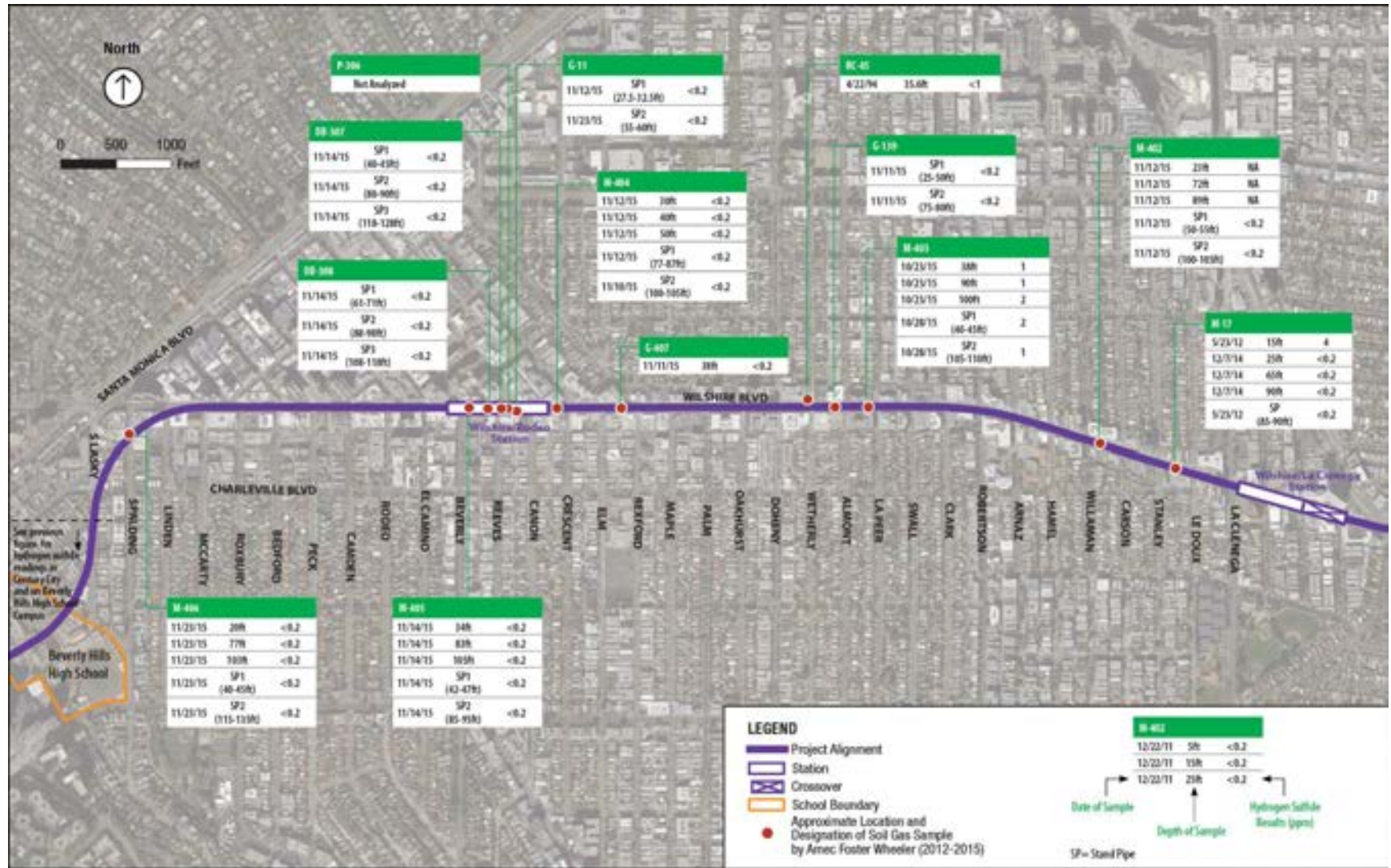
Figure 4-19. Hydrogen Sulfide Readings along Section 2 of the Project, East of Lasky Drive
