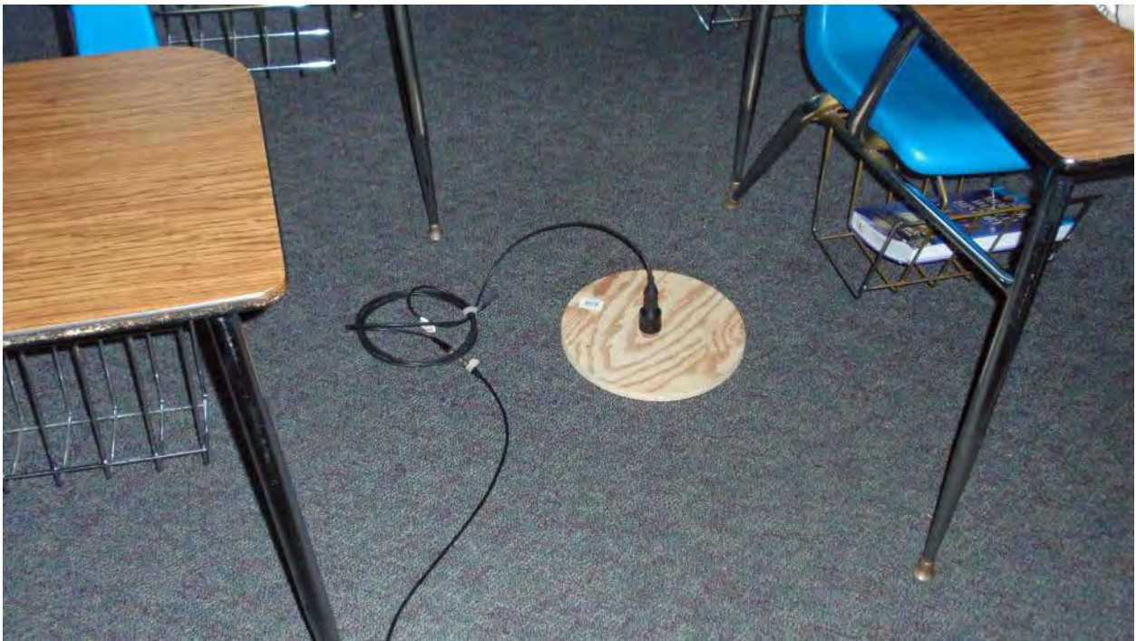
Figure 8-4: Vibration Transducer in Classroom 123
