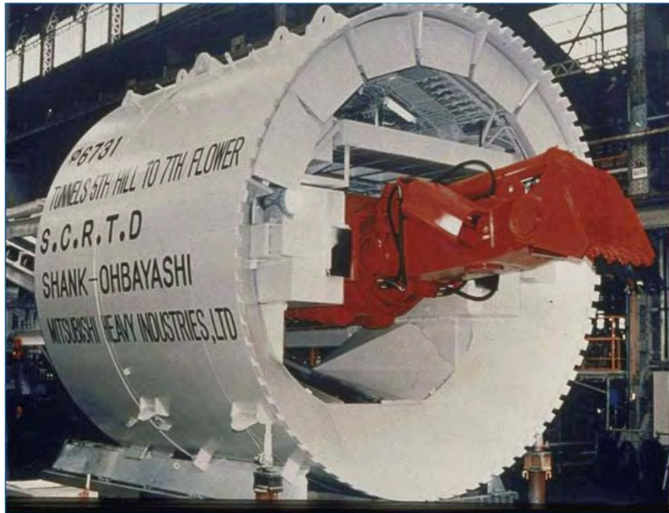
Figure 9-1: Tunnel Shield Used for Metro Segment 1
