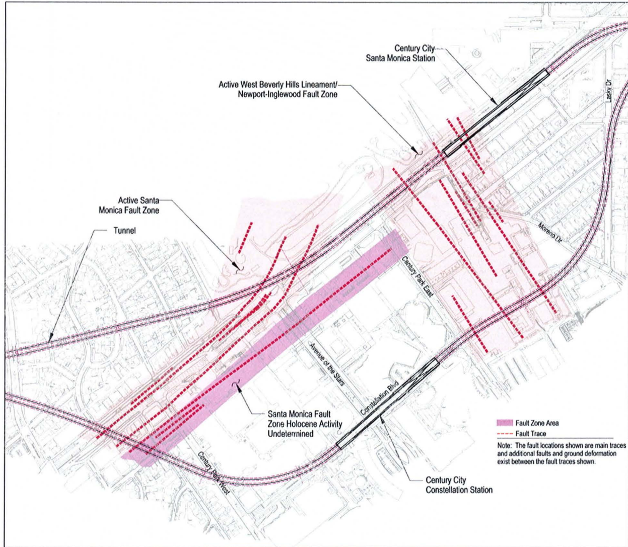
Figure A-14: Fault Zones, Century City, Santa Monica Boulevard Underground Station (Station East of Moreno Drive)
