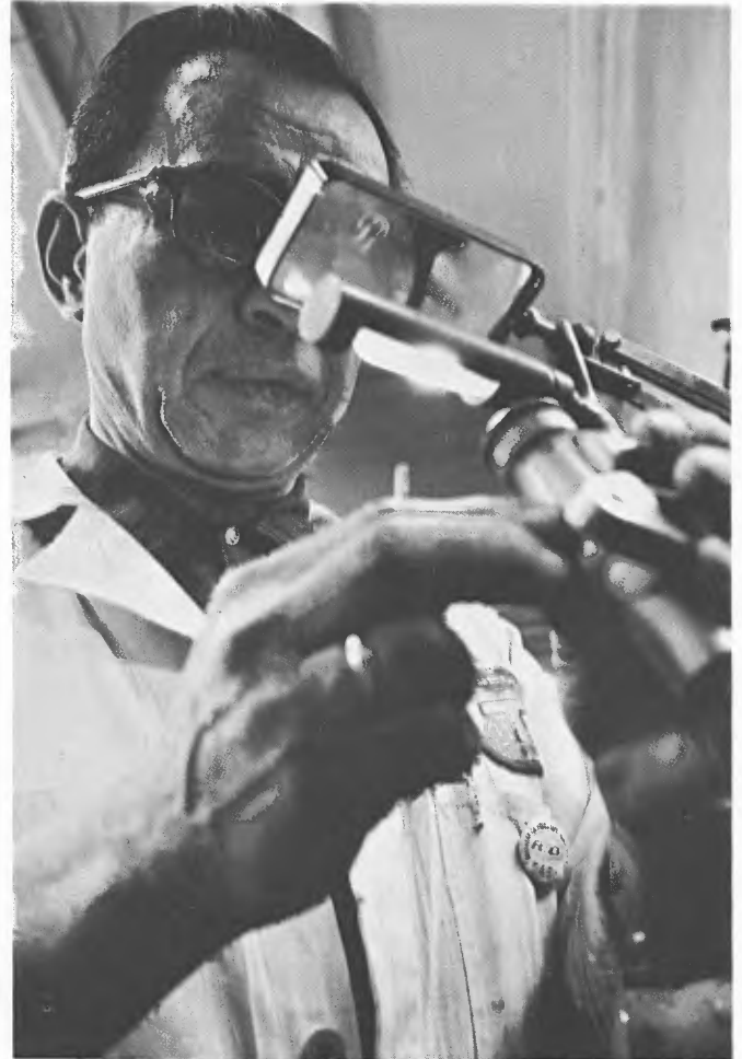
With the aid of a powerful magnifier, machinist Ben Lozano minutely inspects the finish on a coach-leveling valve seat.
