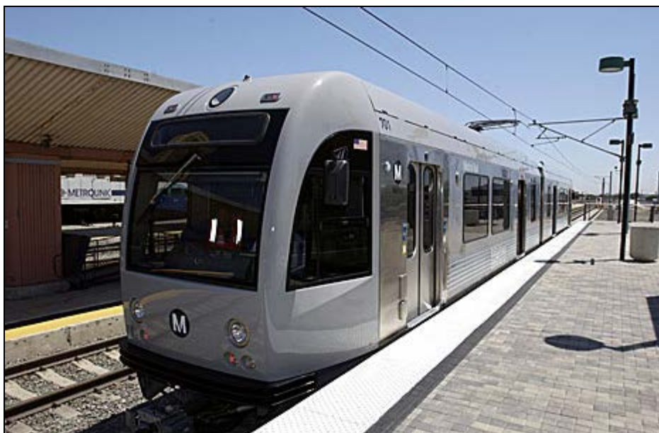
The new 2550 rail car features a stainless steel structure and composite body components.
