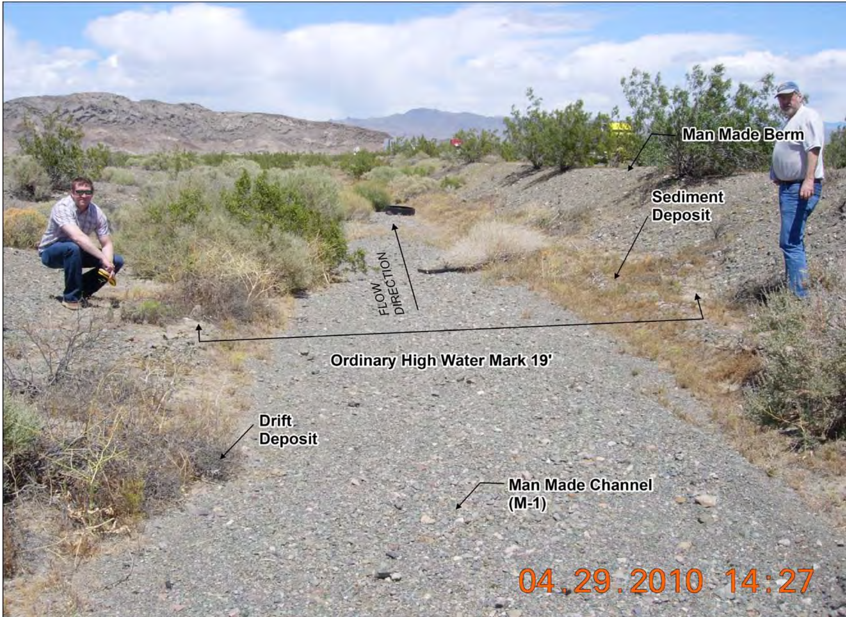
Exhibit A. Figure 9. Typical examples of field indicators of active surface water flow and Ordinary High Water Marks found within ephemerals drainages occurring within the DesertXpress Project Study Area.
