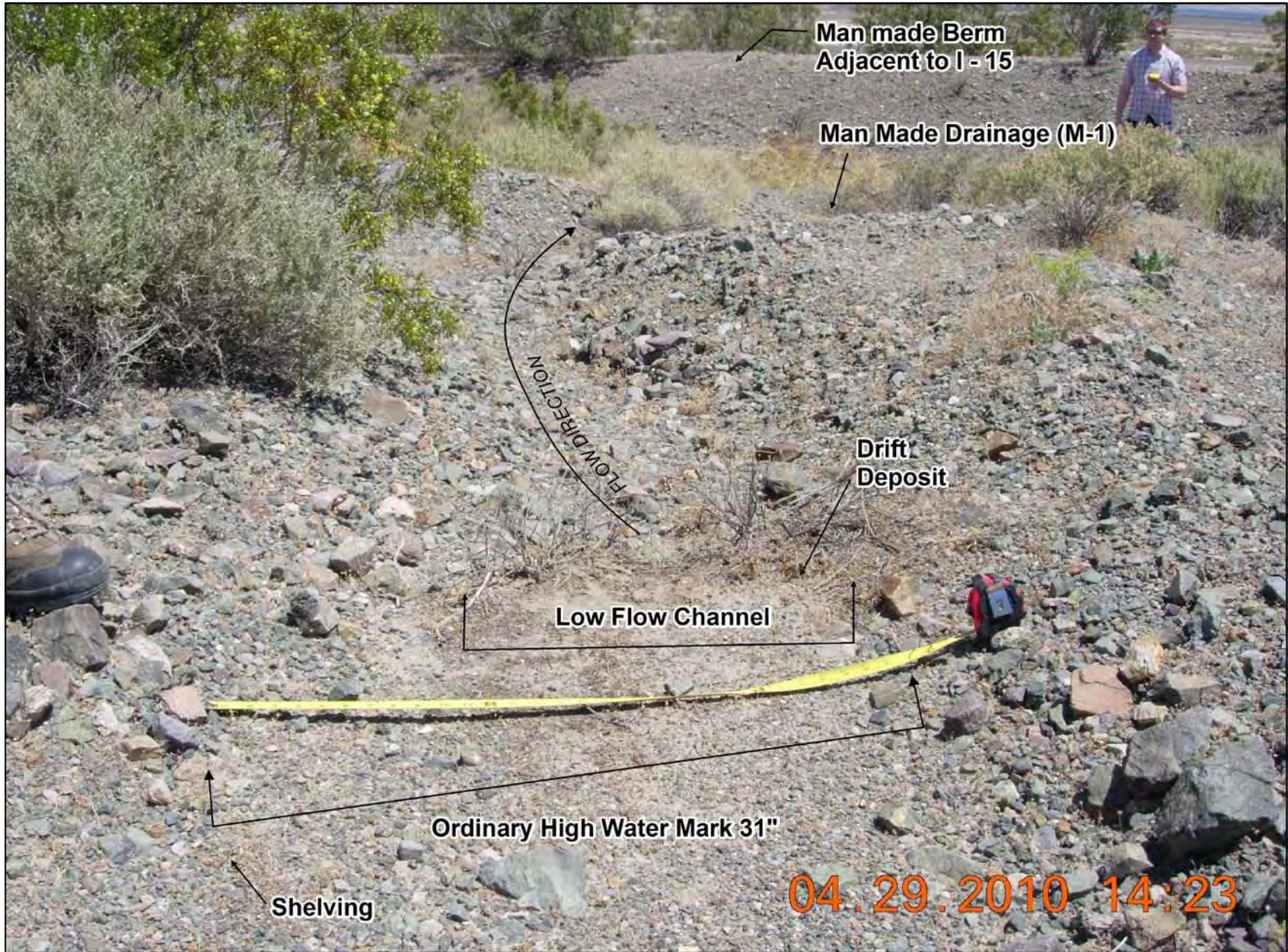
Exhibit A. Figure 7. Typical examples of field indicators of active surface water flow and Ordinary High Water Marks found within ephemerals drainages occurring within the DesertXpress Project Study Area.
