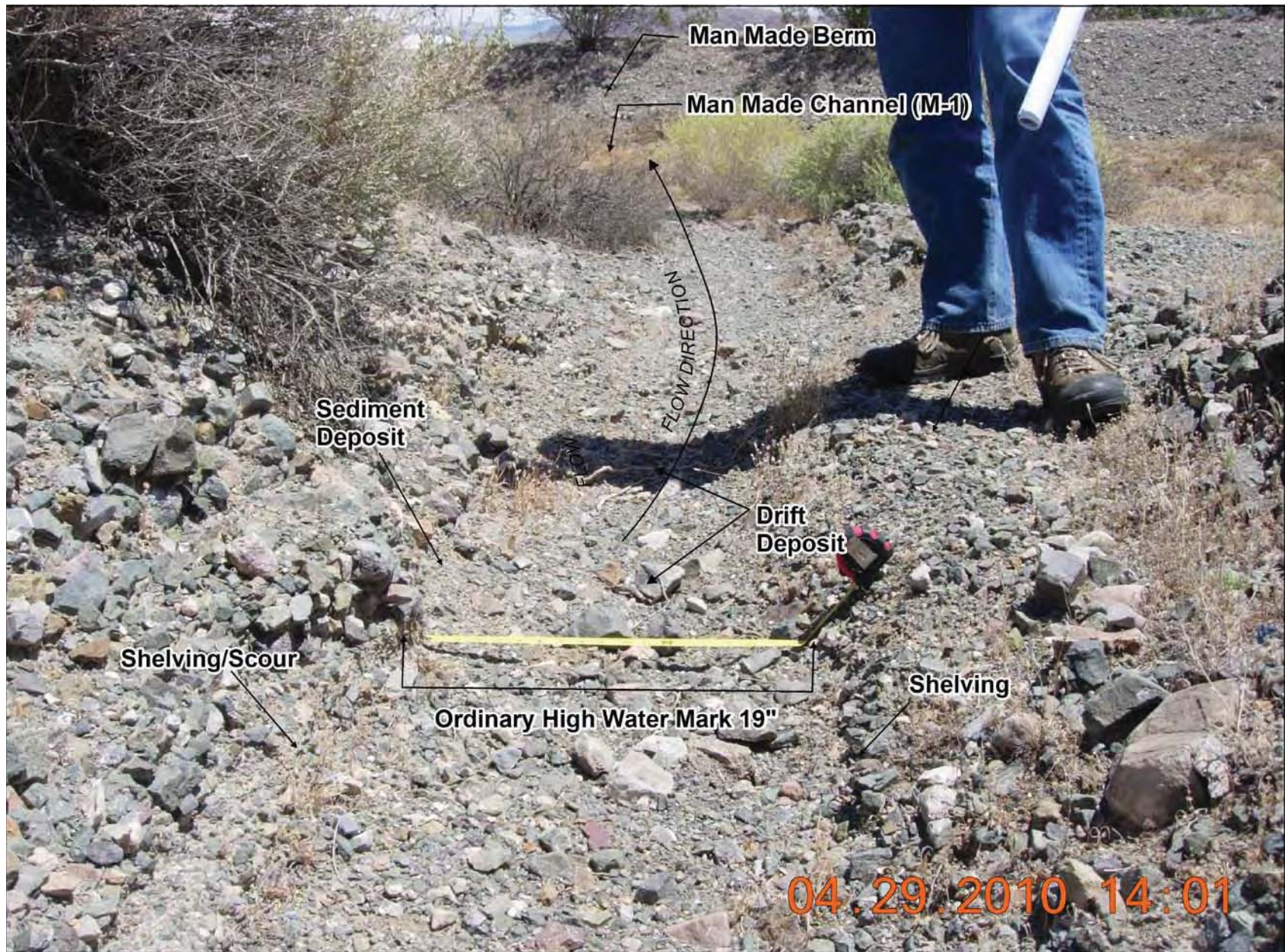
Exhibit A. Figure 5. Typical examples of field indicators of active surface water flow and Ordinary High Water Marks found within ephemerals drainages occurring within the DesertXpress Project Study Area.
