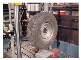
Figure 18. Steel hub and fixture used in the compression test.
