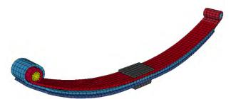
Figure 13. Finite element model of the leaf-spring suspension for a Freightliner FLD 120 tractor.
