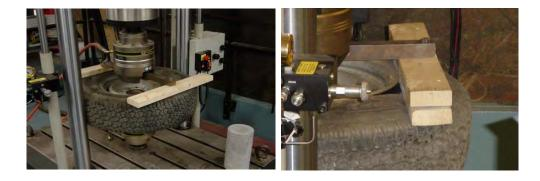
Figure 16. Test setup for the tire de-beading test.
