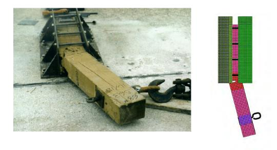
Figure 24. Qualitative comparison of damage in a quasi-static pull-test of a wood guardrail post (left) experiment and (right) simulation.(59)
