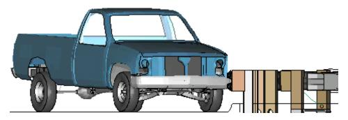
Figure 64. Finite element model for the analysis of the G4(1S) and AASHTO B curb. (146)
