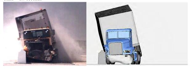
Figure 93. Summary of Phenomenological Events that Occurred during Full-scale Test and Finite Element Model Simulation in Case 4. (continued)
