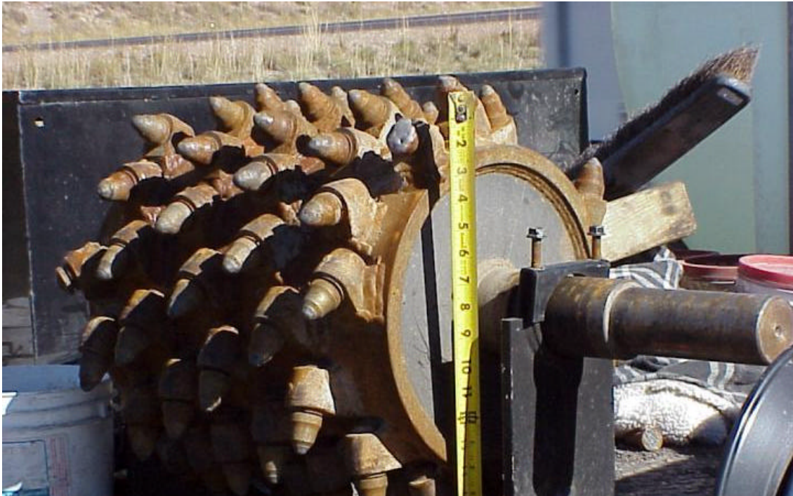
Figure 7. A spare drum for the grinder. The diameter is about 17 inches. By using a drum of smaller diameter grooves could be ground deeper with more flat in between them and still be on 12 inch centers.
