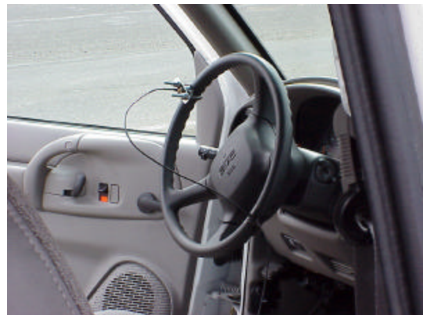
Figure 27. The accelerometer mounted to the top of the steering wheel. It measured vibration levels perpendicular to the plane of the wheel.
