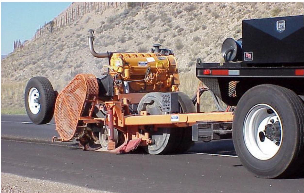
Figure 2. The machine that grinds the standard rumble strips. Inside the large wheel at the front of the machine is the cam that determines the spacing of the rumble strip grooves.
