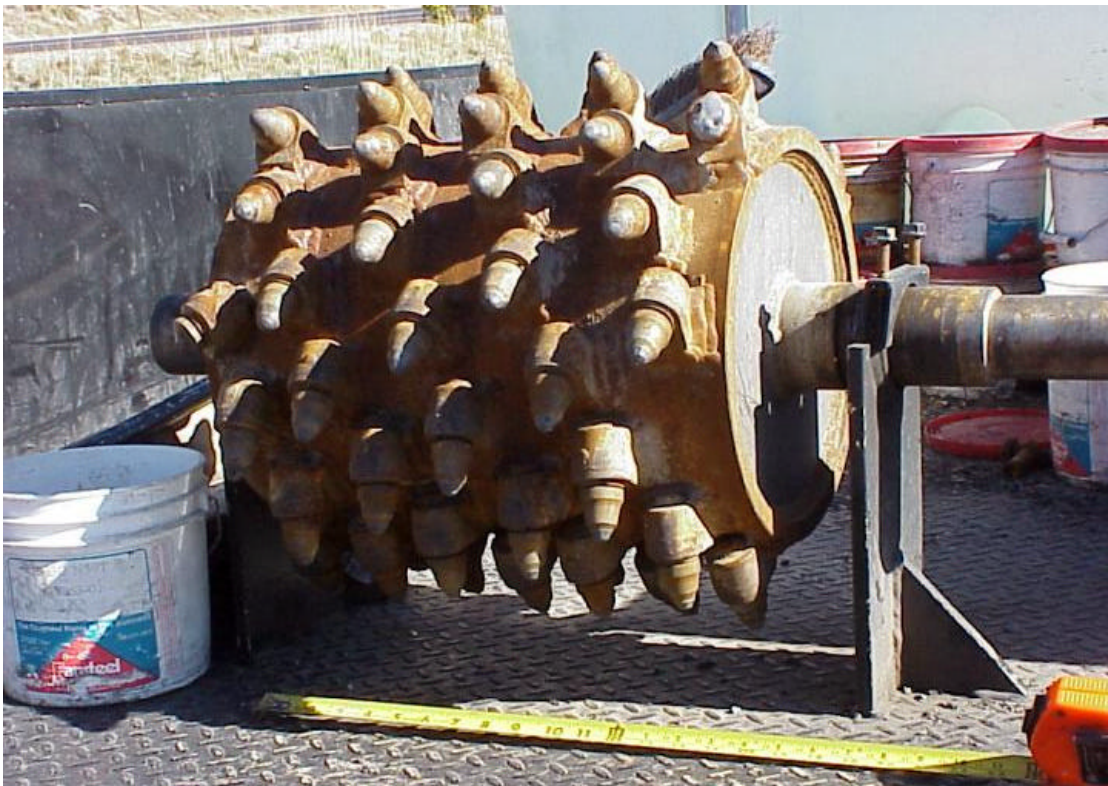
Figure 8. The grinding drum determines the length of the grooves. By leaving some of the end sockets empty, the length of the grooves (the width of the rumble strip) can be varied.
