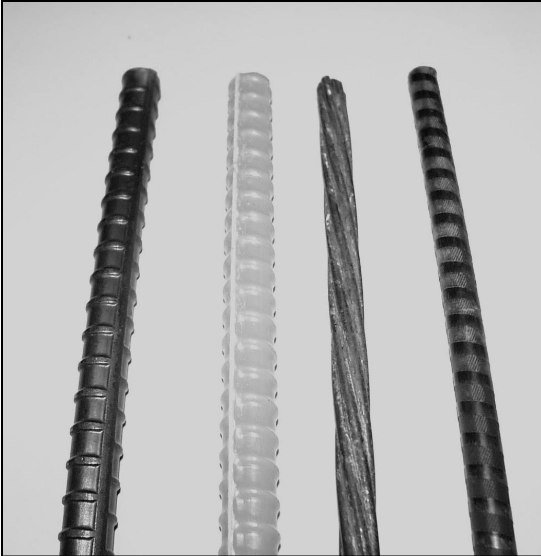
Figure 2.1 Materials used in testing (from left to right): reinforcing steel, C-BAR, prestressing strand, and Leadline
