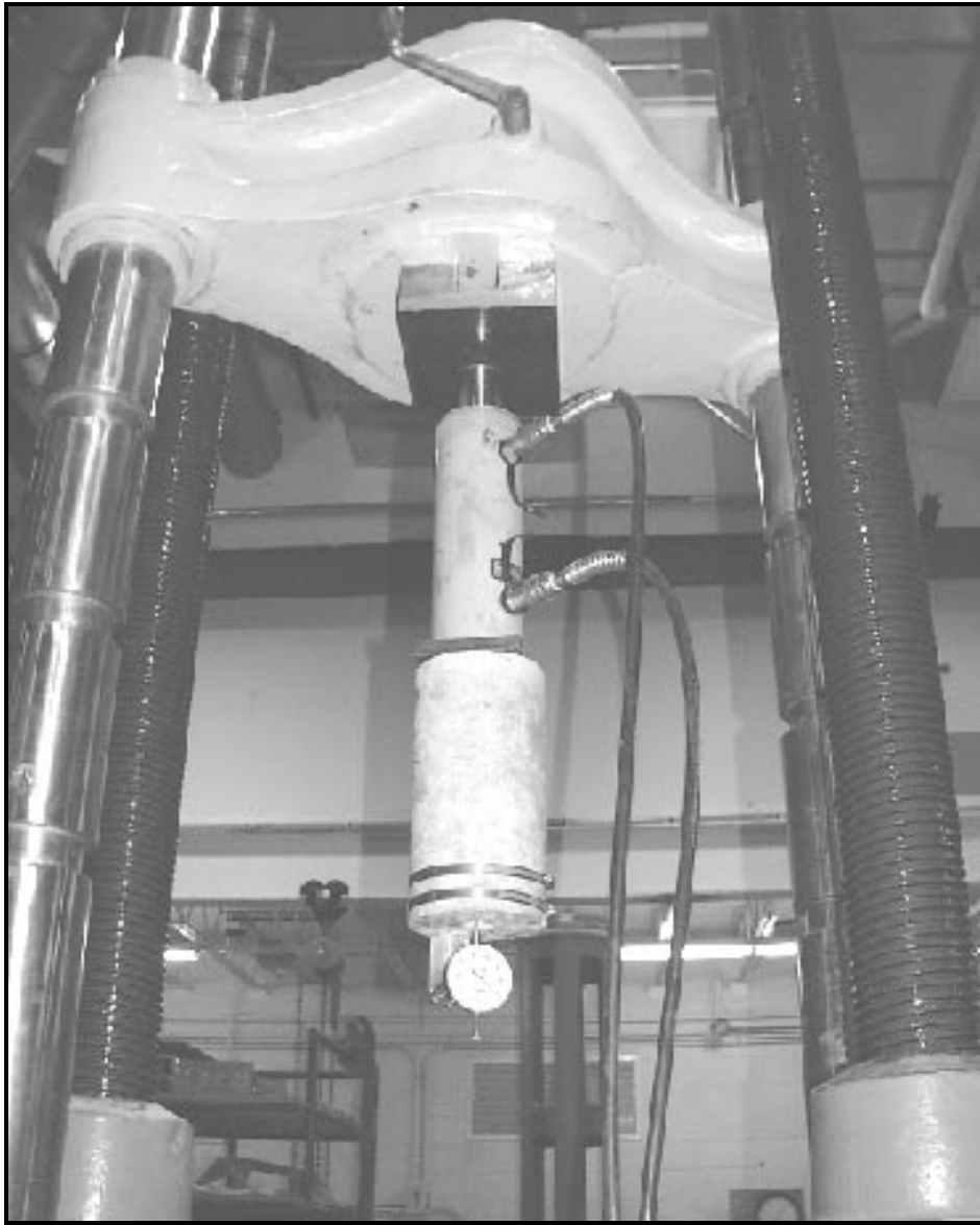
Figure 2.5 FRP bar specimen setup using Universal Testing Machine
