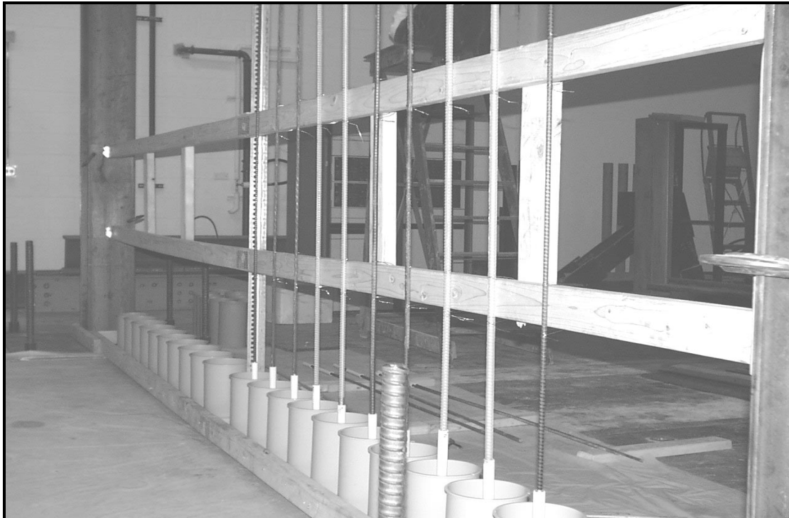
Figure 2.4 Specimen casting setup
