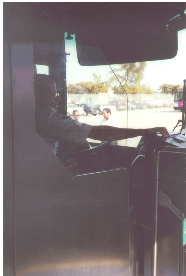
Picture 18 Some MDT operators complain of wrist injuries from customers grabbing transfers from the operators' hands around the Plexiglas panel. A simple design modification—similar to a bank teller's window—may address this concern.
