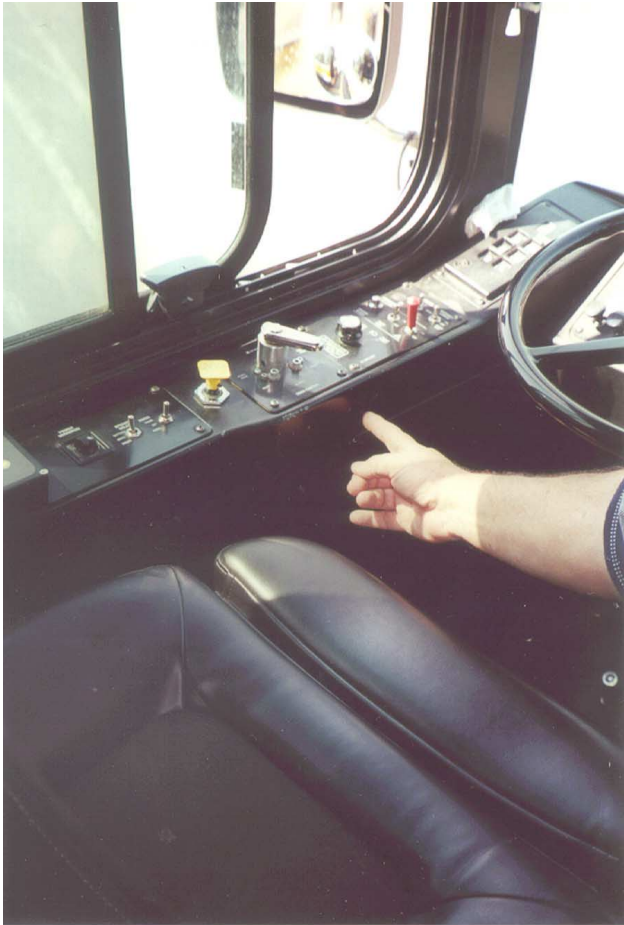
Picture 2 The panic button provides a means for the operator to alert dispatch to a serious problem without using the radio.
