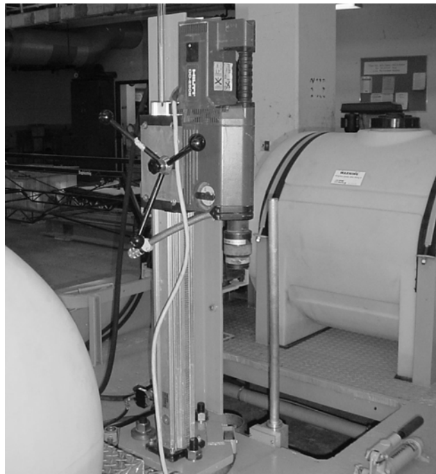
Figure 3-6: Hilti coring device.
