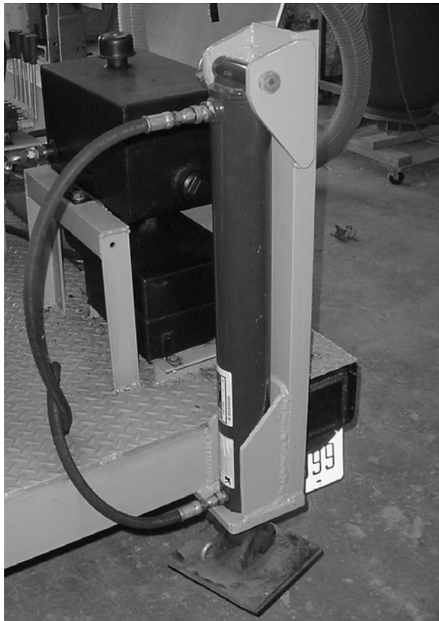
Figure 3-3: One of four hydraulic leveling jacks.
