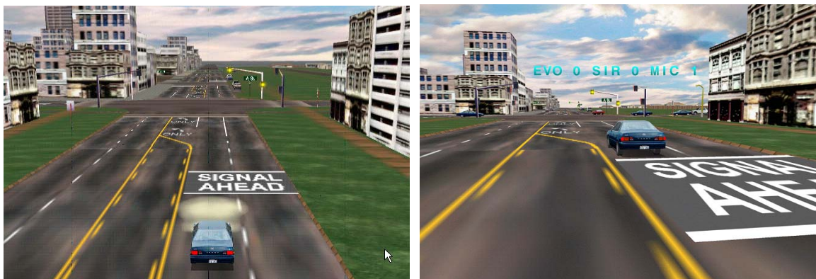
Figure 3-1: Pavement-marking design for reduce red-light running rate
