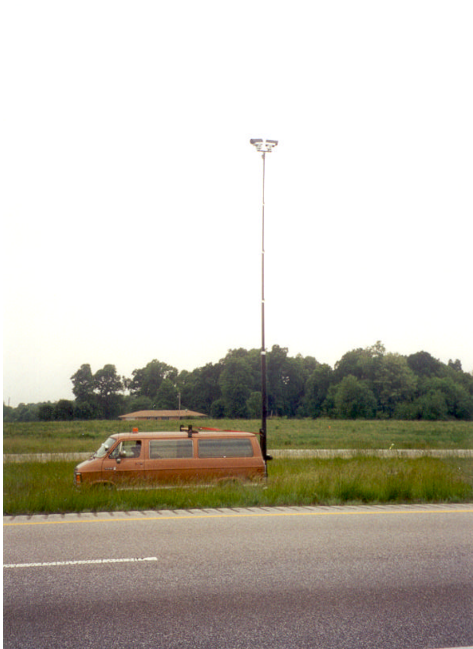
Figure 5.3: The Video detection vehicle (side view) on I-65 near West Lafayette, Indiana
