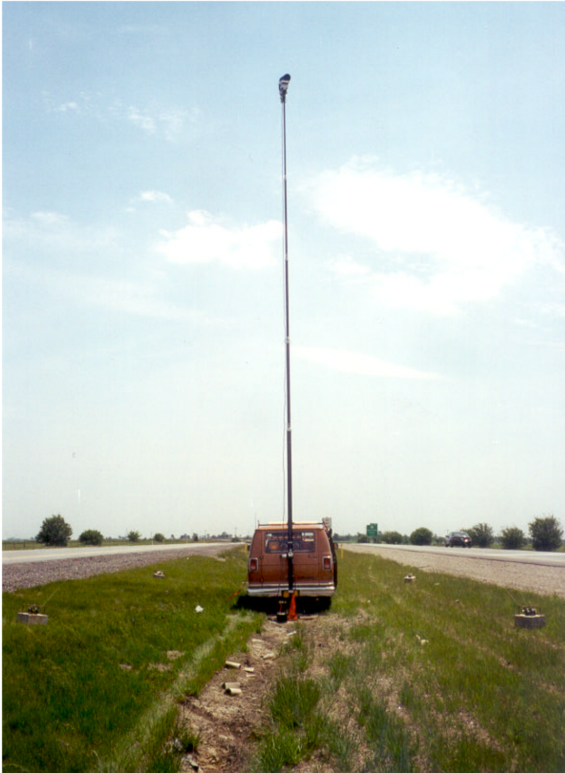
Figure 5.4: The Video detection vehicle (rear view) on I-65 near West Lafayette, Indiana
