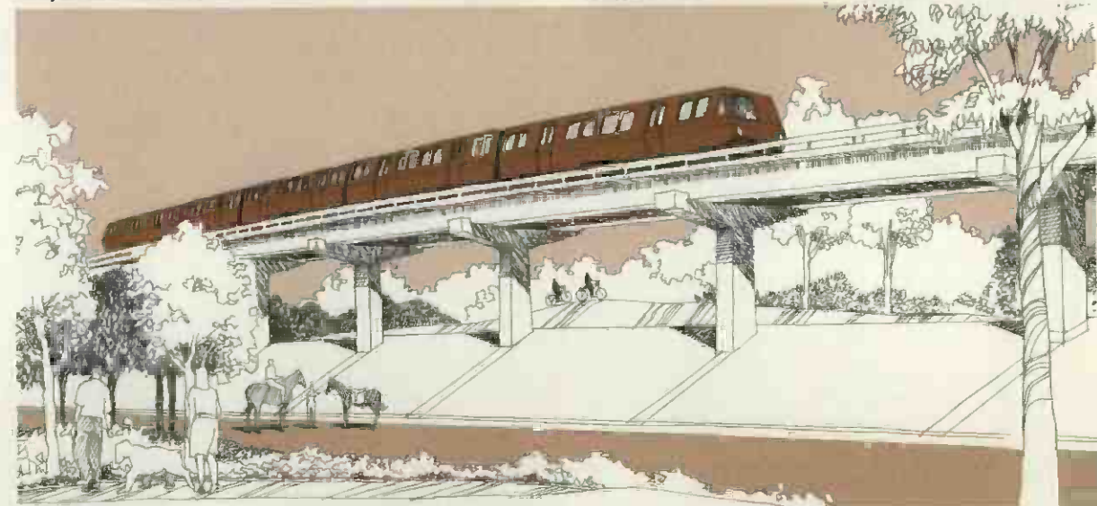
MRT Structure Integrated with Flood Control Channel
