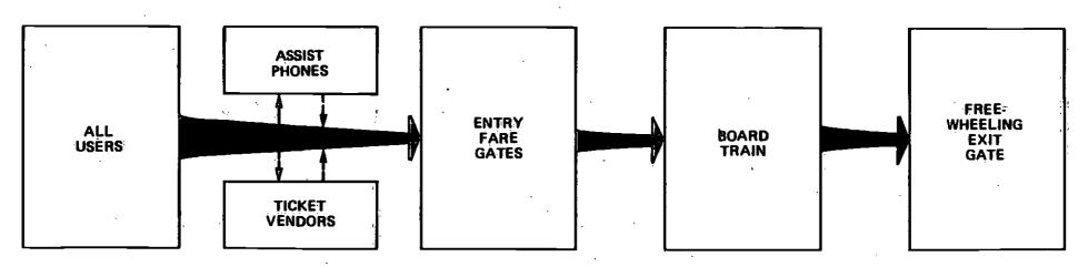
the gates. The agent can also provide informational assistance to patrons. Exit from the station is unrestricted and generally entails crossing the fare control line through a fare gate that free-wheels in the exit direction.
