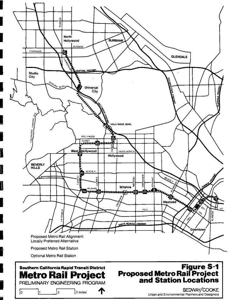
Monica Mountains and proceed to an aerial station at Universal City. Leaving Universal City, the trains would travel on the elevated structure to the terminal station at Lankershim and Chandler Boulevards. The complementary bus network and parking facilities are the same as for the Locally Preferred Alternative.
