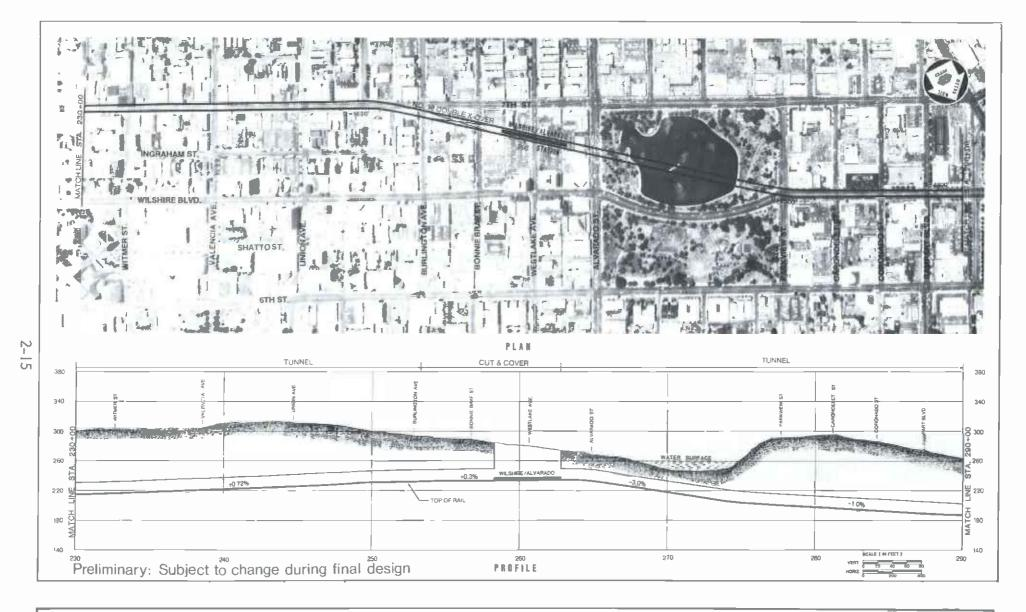
Figure 2.4.5 Alignment for Locally Preferred Alternative
