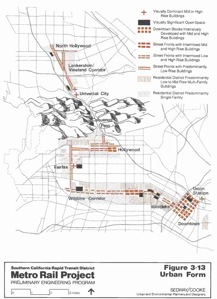
The visual character of each district along the alignment is described to provide a sense of how surface or above ground rail transit facilities may affect the visual setting. Such facilities include park and ride areas, traction power substations, cooling towers, and elevated components of the Aerial Option.
