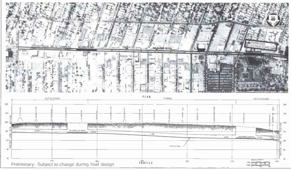
Figure 2.4.9 Alignment for Locally Preferred Alternative
