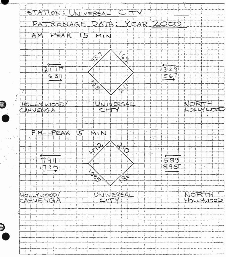
STATION: UNIVERSAL CITY OCCUPANT LOAD - F/LS CRITERIA HEADWAY ASSUMED 32 MIN YEAR 2000 AM PEAK A. PEAK ENTRAINING-4 MISSED HEADWAY ACCUM. 211+957 = 1168 B. LINK LOAD CONTRIBUTIONS: 681 × Y7= 171 2. LINK INBOUND JSE-1200 --1329 + 14= 333 C. TOTAL STATION LOAD 1168 + 1200 = 2368 PM PEAK A. PEAK ENTRAINING - 4 MISSED HEADWAY ACCUM. 186 + 412 = 598 B. LINK LOAD CONTRIBUTIONS! 1. LINK OUTBOUND 449 USE 1200 2. LINK INBOUND 589 × 14 = 148 C. TOTAL STATION LOAD 598+1200 = 1798
