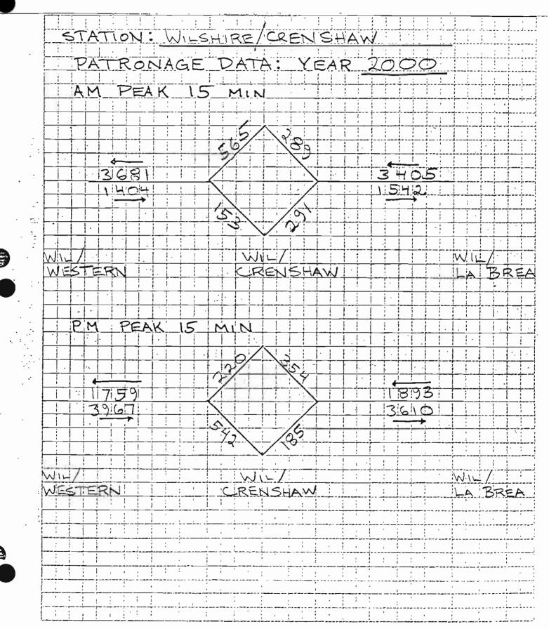
STATION: WILSHIRE/CRENSHAW OCCUPANT LOAD - F/LS CRITERIA HEADWAY ASSUMED 32 MIN YEAR 2000 AM PEAK A. PEAK ENTRAINING-4 MISSED HEADWAY ACCUM. 291 + 565 = 856 B. LINK LOAD CONTRIBUTIONS: 1. LINK OUTBOUND 1404 × 14 = 351 2. LINK INBOUND 3405 \* 14 = 852 C. TOTAL STATION LOAD 856+351+852= 205 PM PEAK A. PEAK ENTRAINING - 4 MISSED HEADWAY ACCUM. 185 + 220 = 405 B. LINK LOAD CONTRIBUTIONS! 1. LINK OUTBOUND 3967 × 1/4 = 992 2. LINK INBOUND 1893 × 14 = 474 C. TOTAL STATION LOAD 405 + 992 + 474 =
