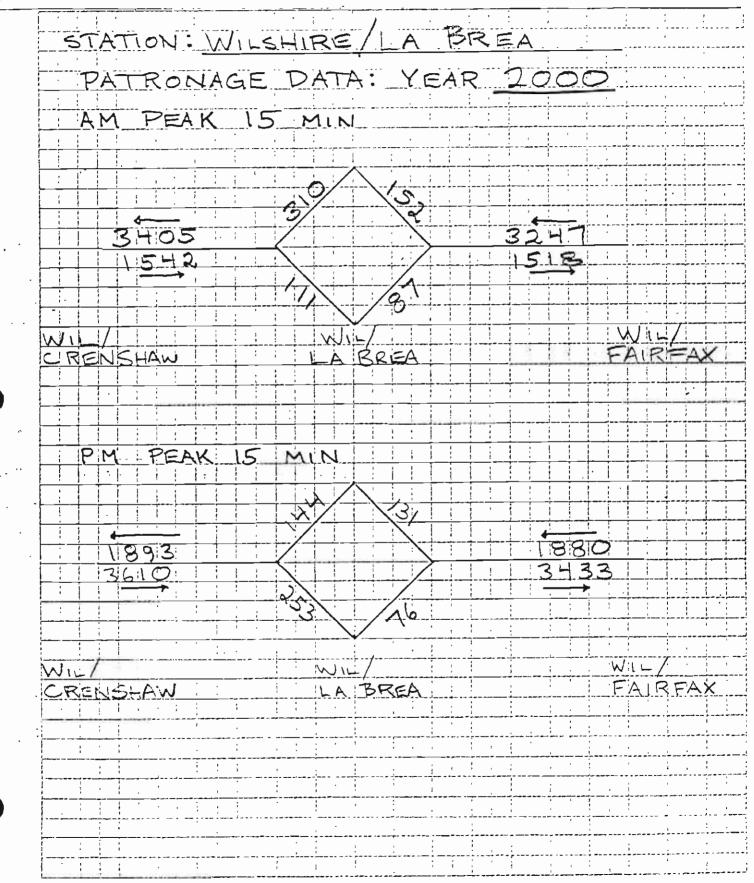
STATION: WILSHIRE/LA BREA OCCUPANT LOAD - F/LS CRITERIA HEADWAY ASSUMED 32 MIN YEAR 2000 AM PEAK A. PEAK ENTRAINING-4 MISSED HEADWAY ACCUM. 87+310= 397 B. LINK LOAD CONTRIBUTIONS: 1. LINK OUTBOUND 1542 × 14 = 386 USE 812/1200 2. LINK INBOUND 3247 × 14 = C. TOTAL STATION LOAD 397+ 1200 = 1597 - ----PM PEAK A. PEAK ENTRAINING - 4 MISSED HEADWAY ACCUM. 76+144 = 220 B. LINK LOAD CONTRIBUTIONS! 1. LINK OUTBOUND 3610× 14 = 903 2. LINK INBOUND 470 C. TOTAL STATION LOAD 1593 220+903+470= 1593
