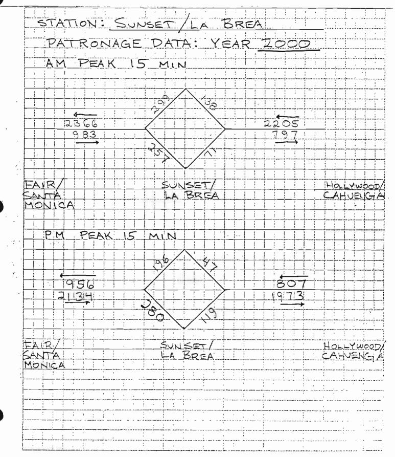
STATION: SUNSET/LA BREA OCCUPANT LOAD - F/LS CRITERIA HEADWAY ASSUMED 31/2 MIN YEAR 2000 AM PEAK A. PEAK ENTRAINING - 4 MISSED HEADWAY ACCUM. 71 + 299 = 370 LINK LOAD CONTRIBUTIONS: 1. LINK OUTBOUND 983×44 = 246 USE 1200 2. LINK INBOUND 2205 × 1/4 = 552 C. TOTAL STATION LOAD 370+1200=15 PM PEAK A. PEAK ENTRAINING - 4 MISSED HEADWAY ACCUM. 119 + 196 = 315 B. LINK LOAD CONTRIBUTIONS! 1. LINK OUTBOUND 2134 × 14 = 534 2. LINK INBOUND 807 \* 44 = 202 C. TOTAL STATION LOAD 315+1200= 1515
