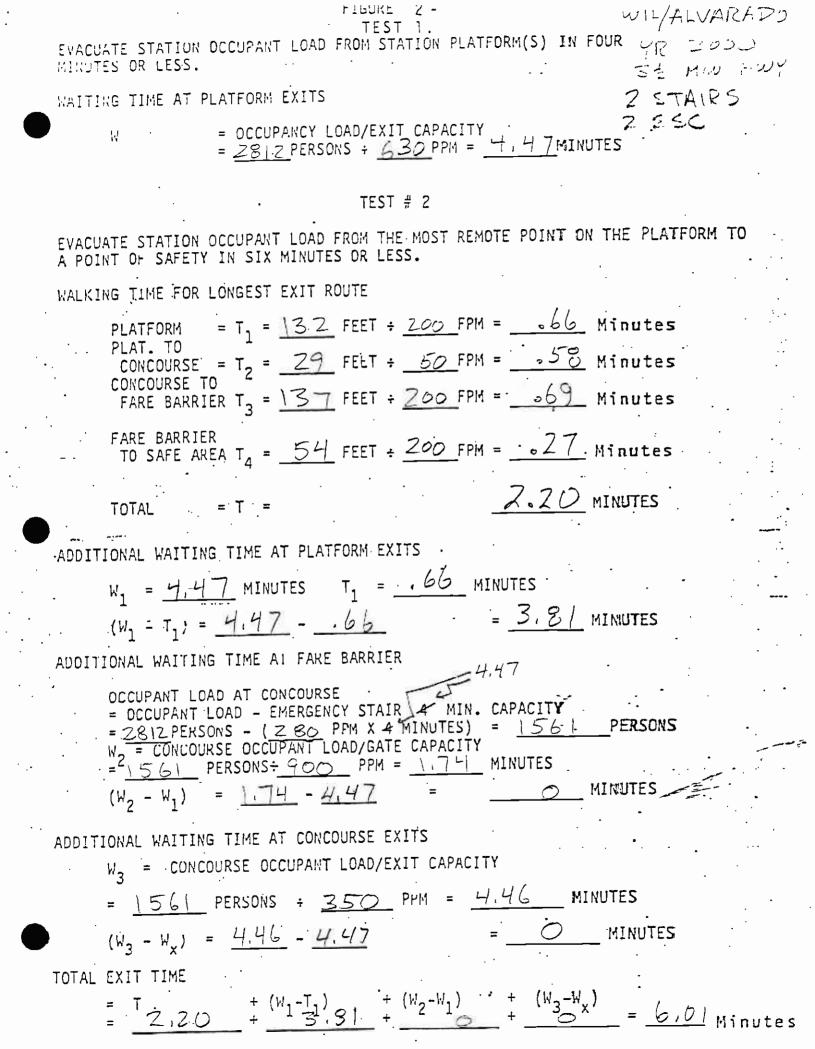
TEST 1.EVACUATE STATION OCCUPANT LOAD FROM STATION PLATFORM(S) IN FOUR Z MIN HWYMINUTES OR LESS.2 STARKSWAITING TIME AT PLATFORM EXITS2 STARKSW= OCCUPANCY LOAD/EXIT CAPACITY= 2531 PERSONS + 630 PPM = 4.02 MINUTES
