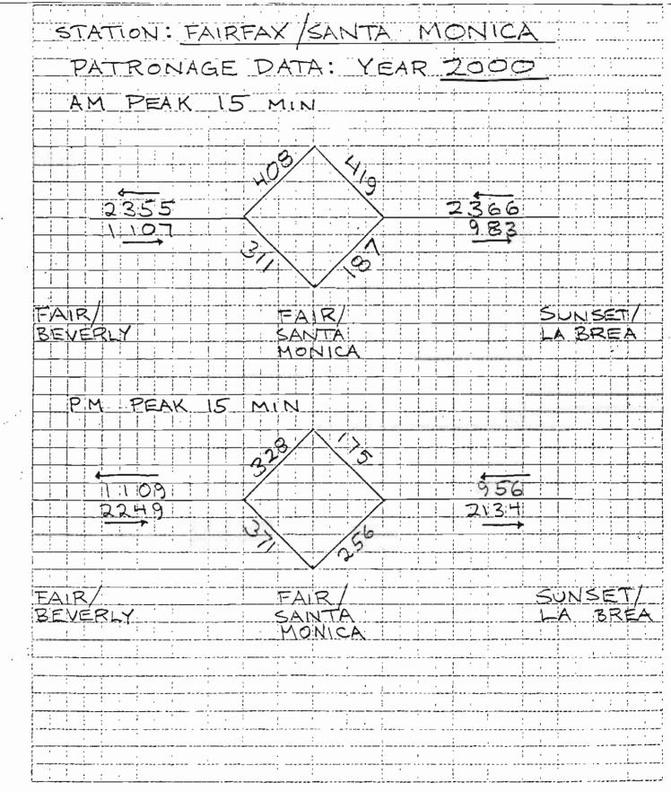
STATION: FAIRFAX/SANTA MONICA OCCUPANT LOAD - F/LS CRITERIA HEADWAY ASSUMED 3/2 MIN YEAR 2000 AM PEAK A. PEAK ENTRAINING-4 MISSED HEADWAY ACCUM. 187+408= 595 B. LINK LOAD CONTRIBUTIONS: 1. LINK OUTBOUND 277 2. LINK INBOUND JUSE 1200 2366 × Y4 = 592 C. TOTAL STATION LOAD 1795 PM PEAK A. PEAK ENTRAINING - 4 MISSED HEADWAY ACCUM. 256 + 328 = 584 B. LINK LOAD CONTRIBUTIONS! 1. LINK OUTBOUND 2249 × 1/4 = 563, USE 1200 LINK INBOUND 956 \* 14 = 239 C. TOTAL STATION LOAD 584 + 1200 = 1784
