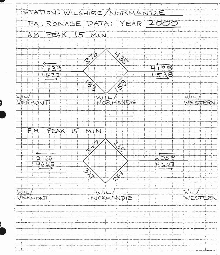
STATION: WILSHIRE/NORMANDIE OCCUPANT LOAD - F/LS CRITERIA HEADWAY ASSUMED 312 MIN YEAR 2000 AM PEAK A. PEAK ENTRAINING-4 MISSED HEADWAY ACCUM. 159+376 = 535 B. LINK LOAD CONTRIBUTIONS: 1622 × 14 = 406 2. LINK INBOUND 4198 × 14= 1050 TOTAL STATION LOAD 535 + 406 + 1050 = 1991 PM PEAK A. PEAK ENTRAINING - 4 MISSED HEADWAY ACCUM. 269 + 347 = 616 B. LINK LOAD CONTRIBUTIONS! 1. LINK OUTBOUND 4665 × 14 = 1167 2. LINK INBOUND 2054 × 1/4 = 514 C. TOTAL STATION LOAD 616 + 1167 + 514 = 2297
