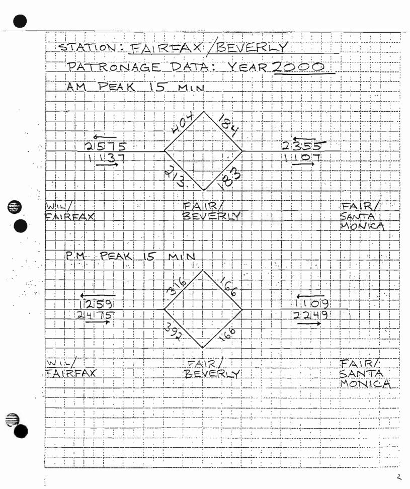
STATION: FAIRFAX/BEVERLY OCCUPANT LOAD - F/LS CRITERIA HEADWAY ASSUMED 31/2 MIN YEAR 2000 AM PEAK A. PEAK ENTRAINING-4 MISSED HEADWAY ACCUM. 183+404 = 587 B. LINK LOAD CONTRIBUTIONS: 1. LINK OUTBOUND 285, 2. LINK INBOUND USE 1200-2355 \* 14 = 589 C. TOTAL STATION LOAD 587+1200=1787 PM PEAK A. PEAK ENTRAINING - 4 MISSED HEADWAY ACCUM. 166 + 316 = 482 B. LINK LOAD CONTRIBUTIONS! 1. LINK OUTBOUND 2475 × 14 = 619 278 USE 1200 2. LINK INBOUND C. TOTAL STATION LOAD 482+1200 = 1682
