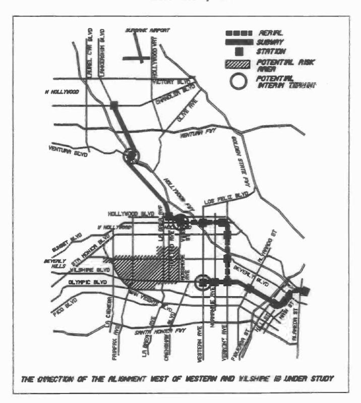
This line is planned to be the core element of a regional rail rapid transit system. In addition to the planned 20-mile line, two future extensions of the Metro Rail system have been identified as part of the regional rail rapid transit system. These future extensions may involve surface as well as subway or aerial segments.
