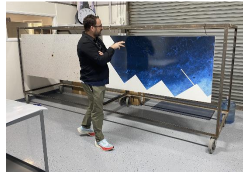
Grand Av Arts/Bunker Hill Station Factory Inspection of Porcelain Enamel Steel Artwork Panels
